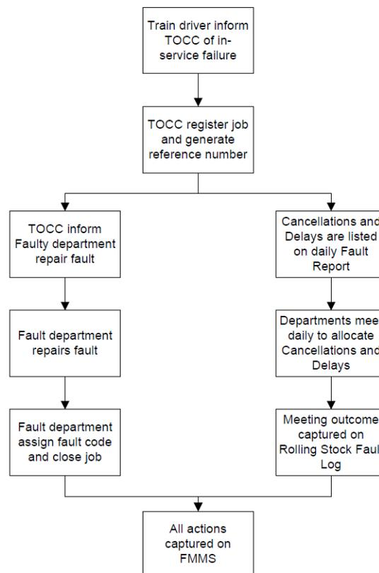
Figure 4 : In-Service Failure Process Flow
