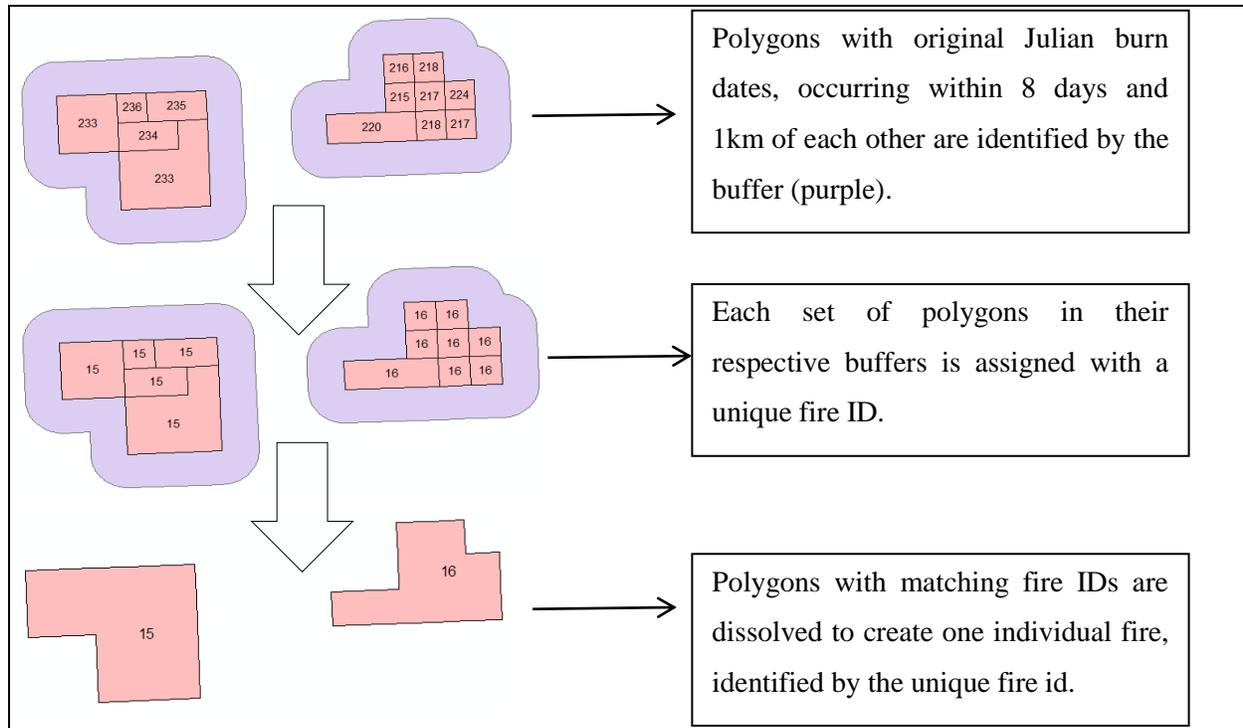
Figure 3.5 Process of identifying individual fires using the 8 day/1 km algorithm
