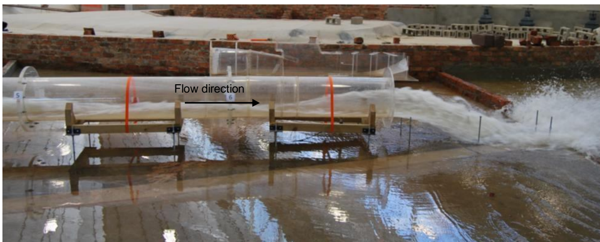
Photograph 50: Free surface flow at outlet for 20% gate opening for modification 4
