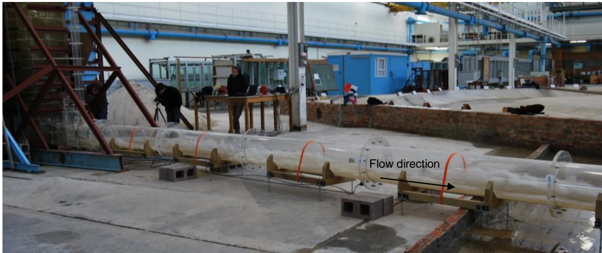
Photograph 49: Free surface flow upstream for 20% gate opening for modification 4
