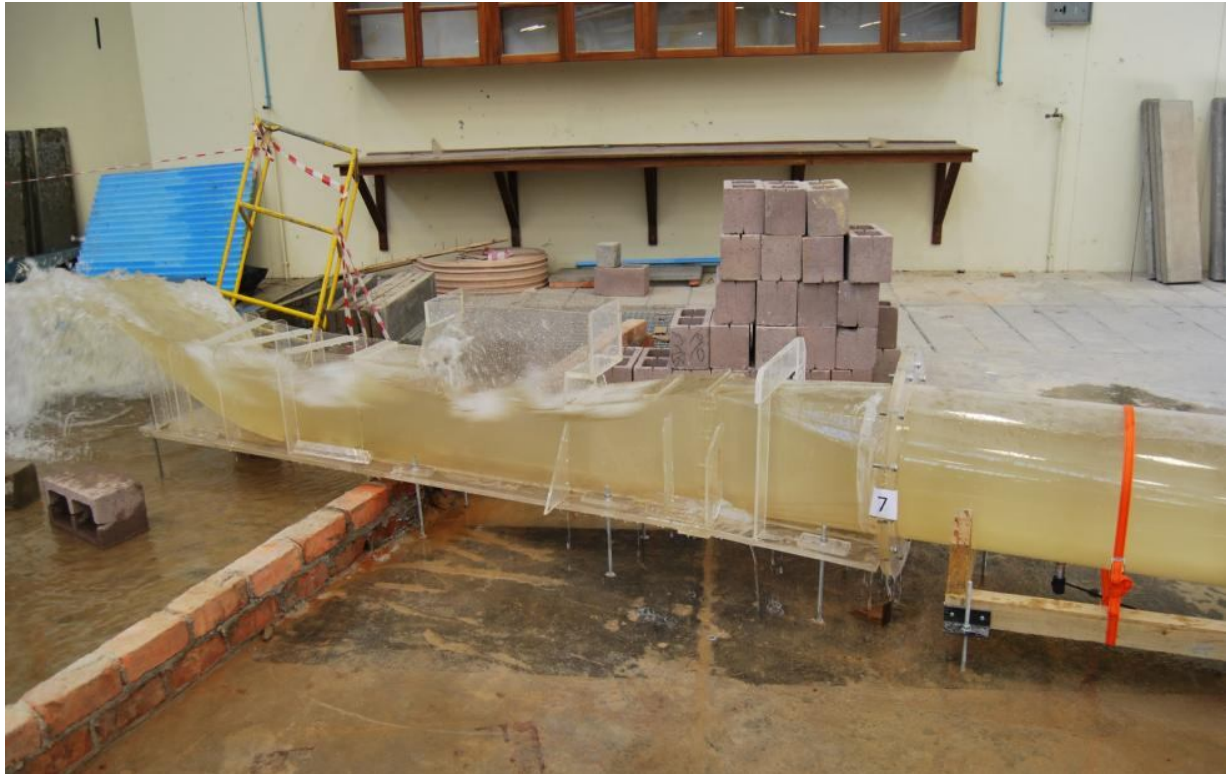
Photograph 3: Radial gate chamber and ski-jump at end of outlet conduit
