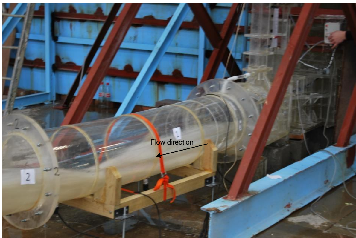
Photograph 44: Spray flow occurred at small gate openings
