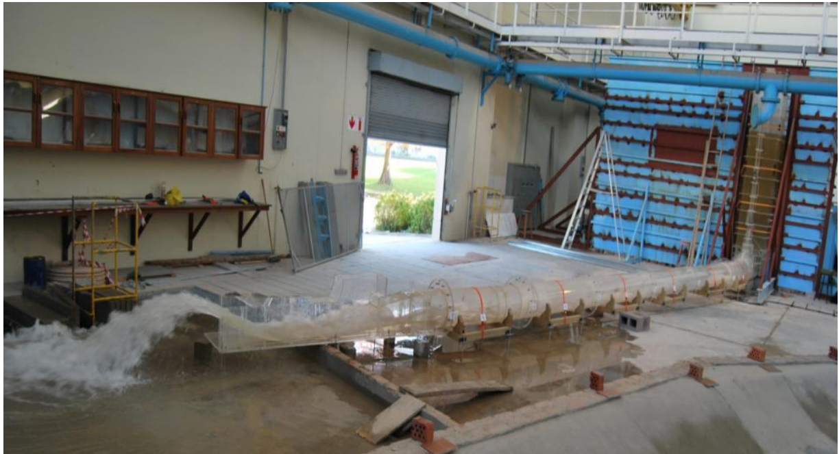
Photograph 1: Layout of Berg River Dam Model
