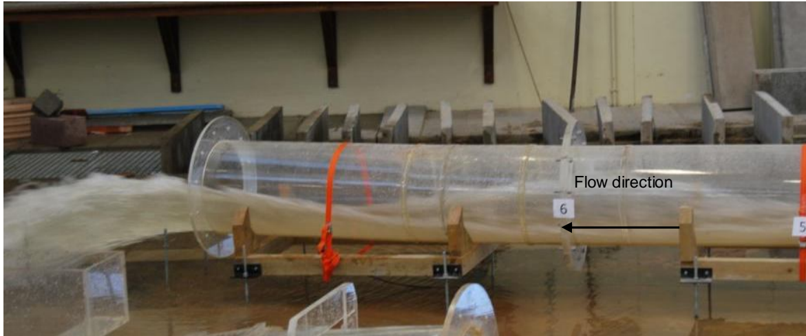
Photograph 42: Free surface flow at outlet for a 40% gate opening for modification 4
