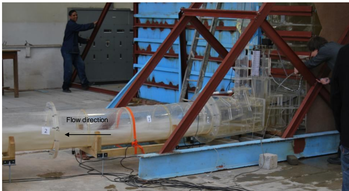
Photograph 41: Free surface flow at emergency gate for a 40% gate opening for modification 4
