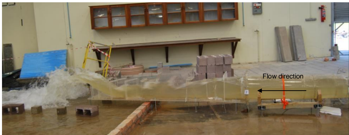
Photograph 36: Flow conditions at outlet (all excl. modification 4)
