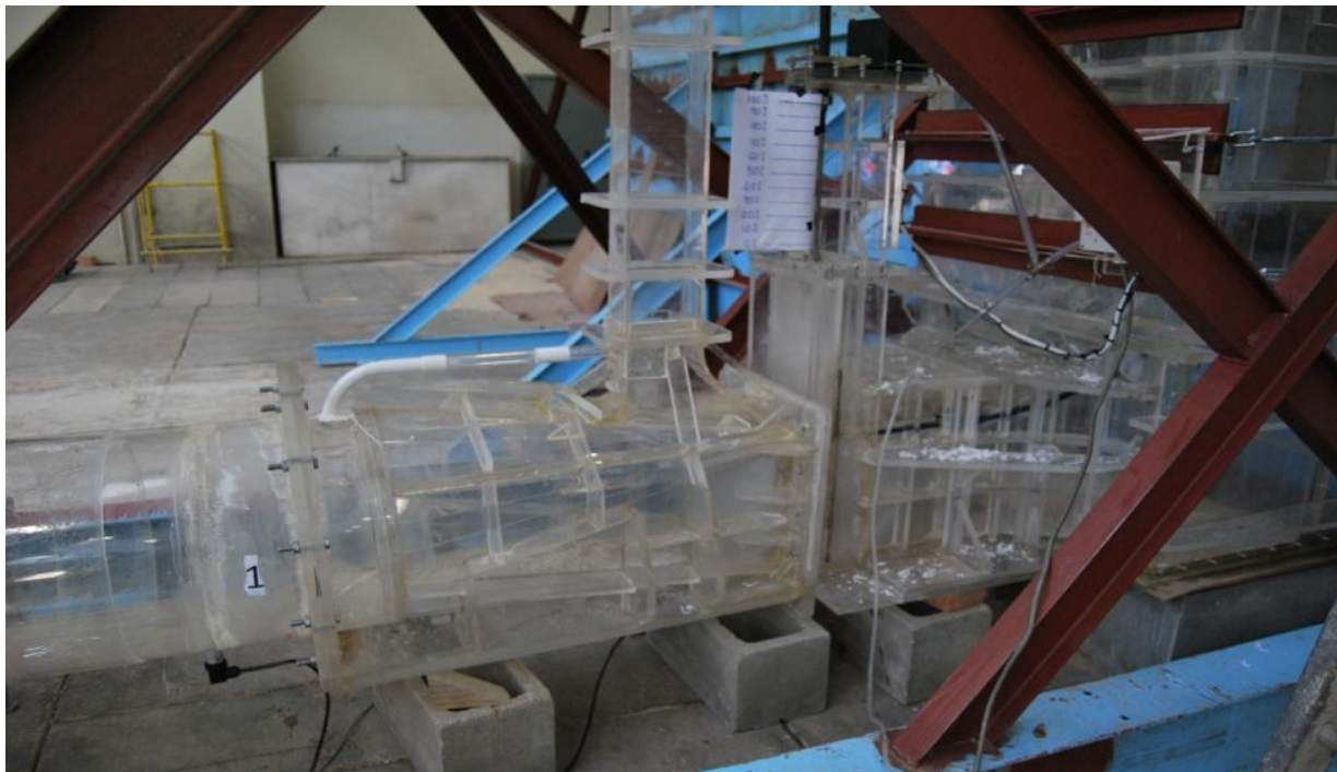
Photograph 2: Emergency gate, base of air shaft and outlet conduit
