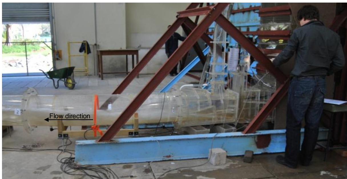
Photograph 37: Free surface flow at emergency gate for a 50% gate opening for modification 4
