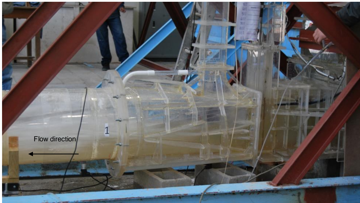
Photograph 29 Free surface flow at emergency gate for 70% gate opening (modification 4)
