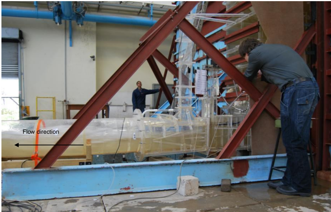
Photograph 24: Free surface flow at emergency gate at 80% gate opening for modification 4
