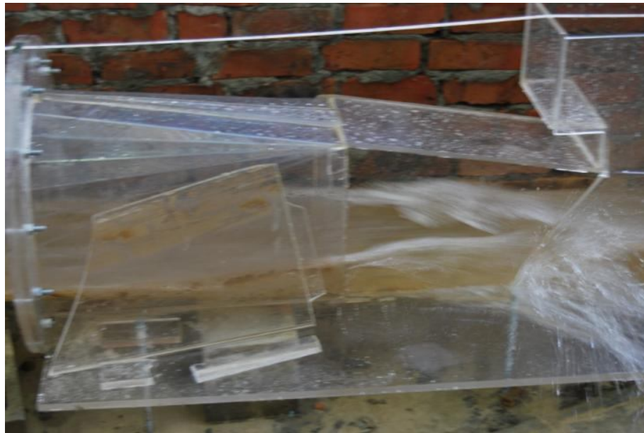
Figure 6.2: Failed radial gate chamber
