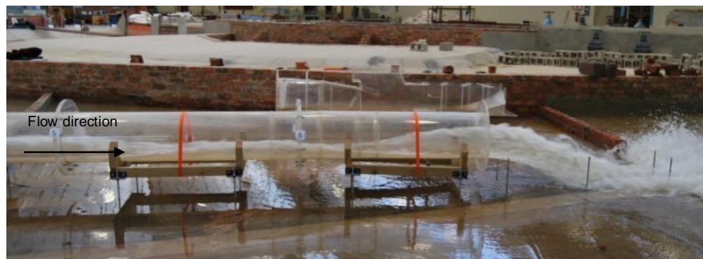
Photograph 10: Modification 4 – ski-jump and radial gate chamber removed
