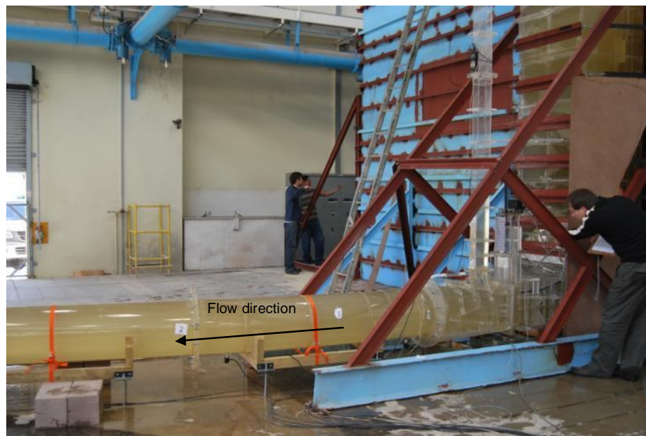
Photograph 21: Pressurised flow downstream of emergency gate – excl. modification 4
