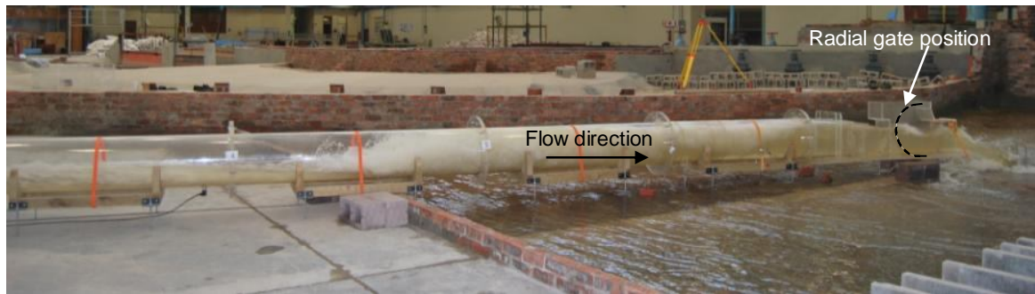
Photograph 43: Hydraulic jump “trapped” by tapered section of radial gate chamber
