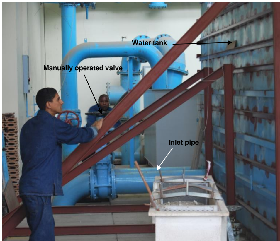
Figure 3.4: Model inlet pipe and valves
