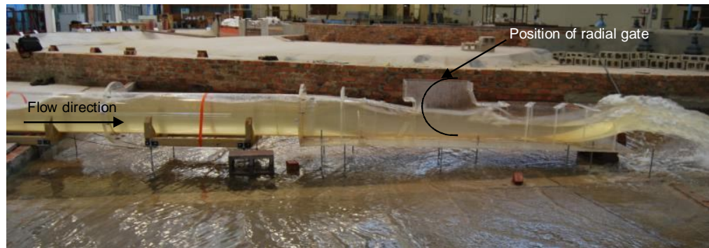
Photograph 9: Modification 3 – second bend removed
