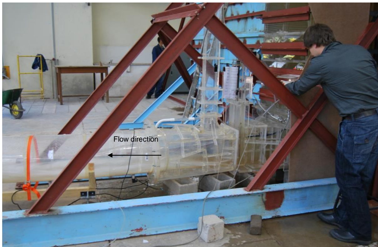
Photograph 45: Free surface flow at emergency gate for a 30% gate opening for modification 4
