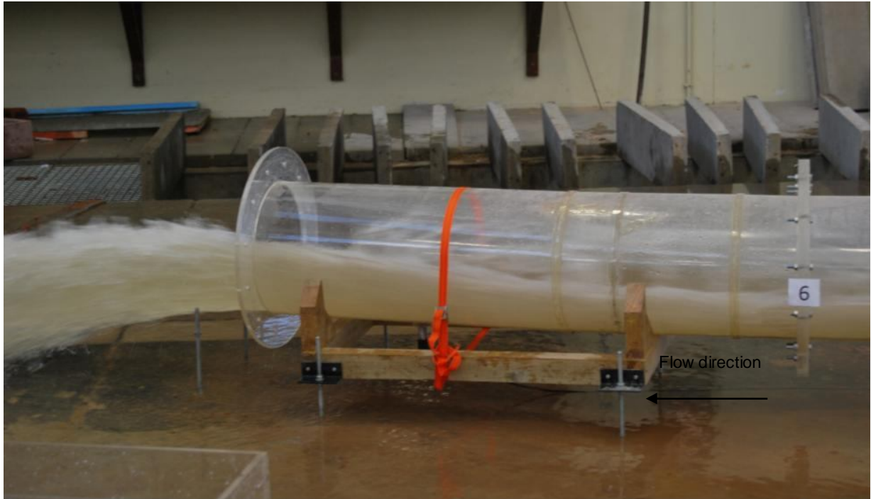
Photograph 30: Free surface flow downstream for 70% gate opening (modification 4)
