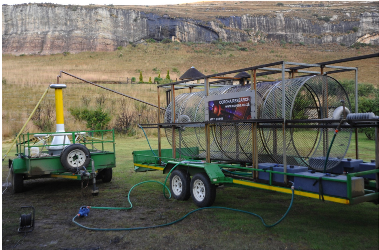
Figure 5.10 Mobile Corona Cage equipped with water tanks, pump and sprayers (Clarens 1900 m above sea level)
