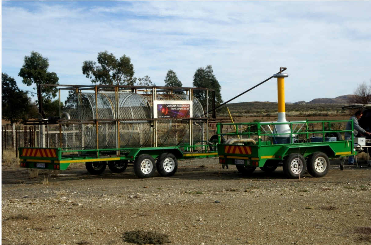
Figure 4.6 Mobile corona cage and AC/DC source
