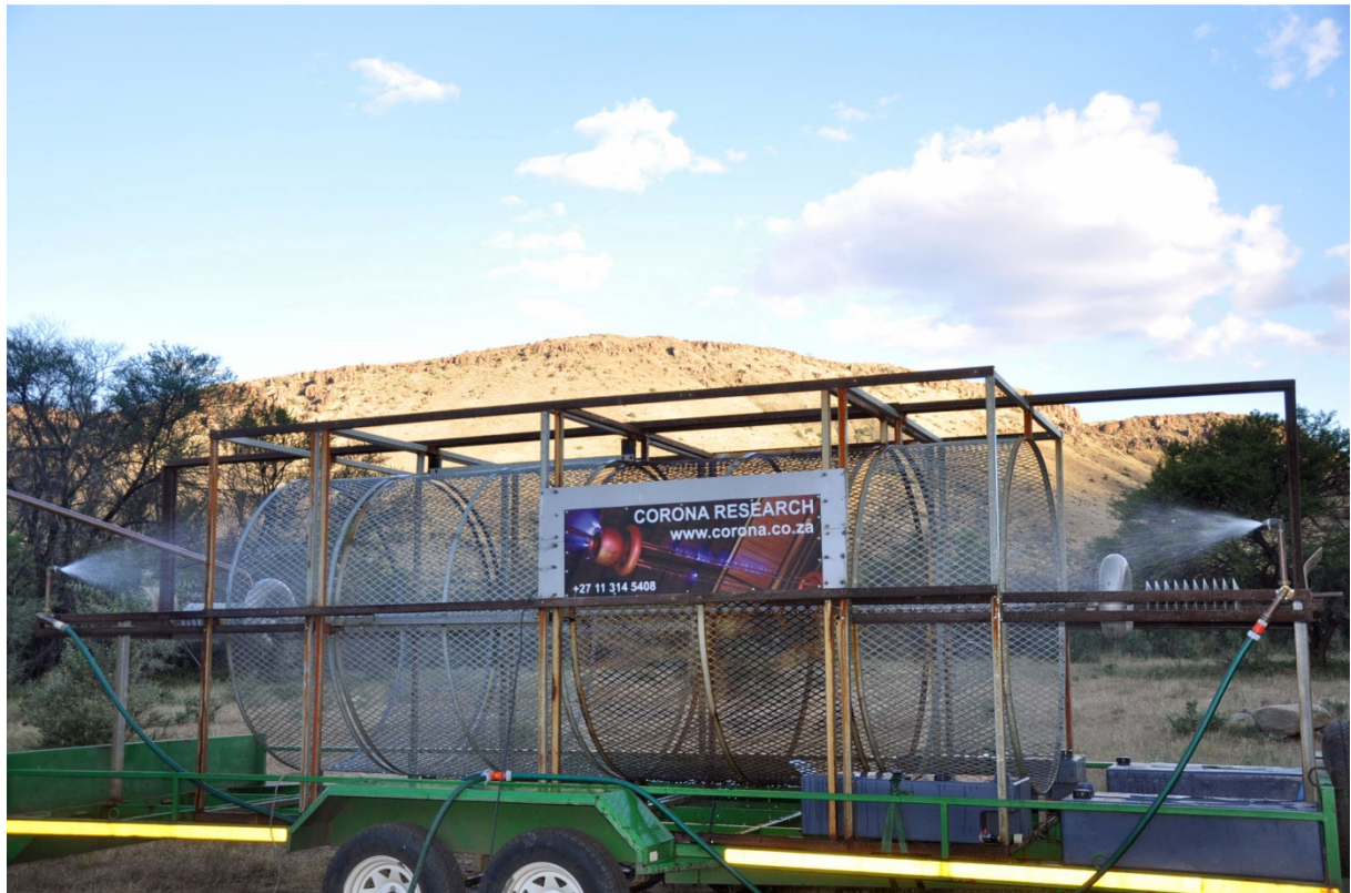
Figure 5.11 Mobile Corona Cage during a wet test (2 mm/min)
