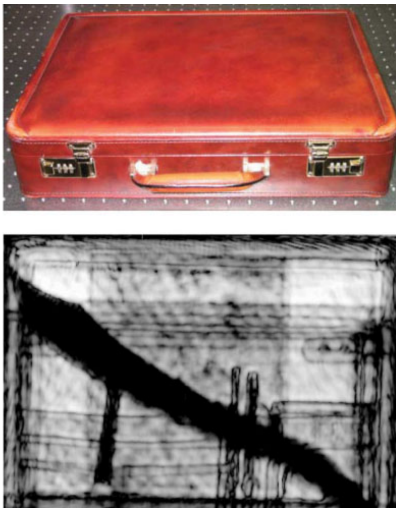
Figure 1.2: An image made of a knife, seen in the lower image, contained in a briefcase. The image was made by constructing an image based on the informations gathered by detector gathering radiation at 0.2 THz. Taken from [4].
