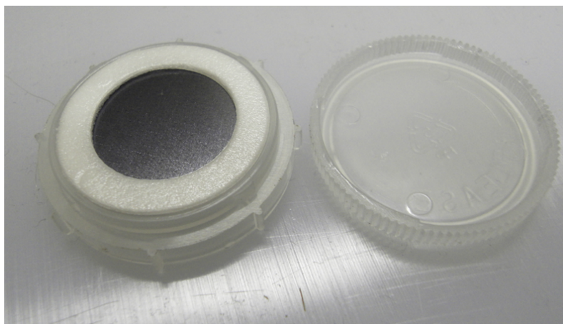
Figure 5.3: The infrared low pass optical filter in its plastic holder.
