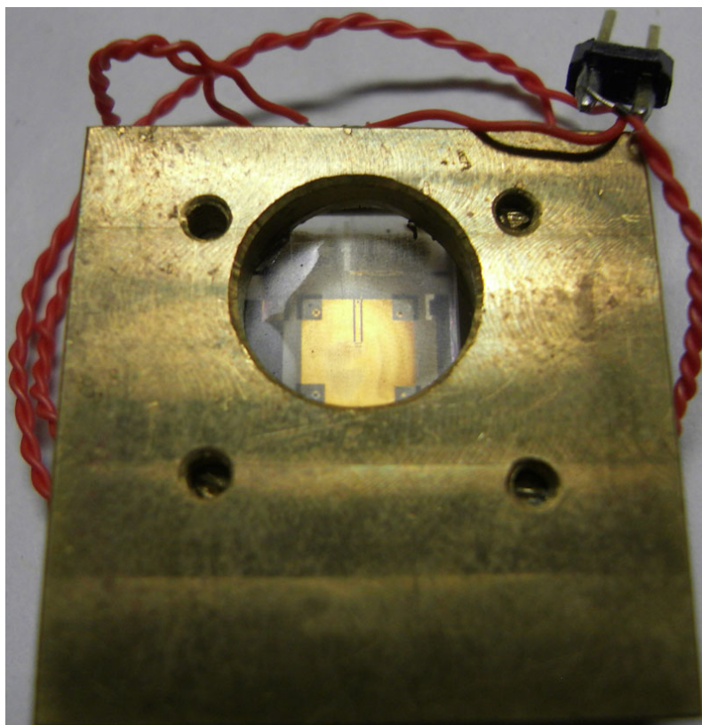
Figure 7.9: The underside of an MgO substrate. The gold ground plane and coplanar waveguide can be seen inside the circular hold in the brass plate. The twin slot antenna is located in the centre of the gold square.
