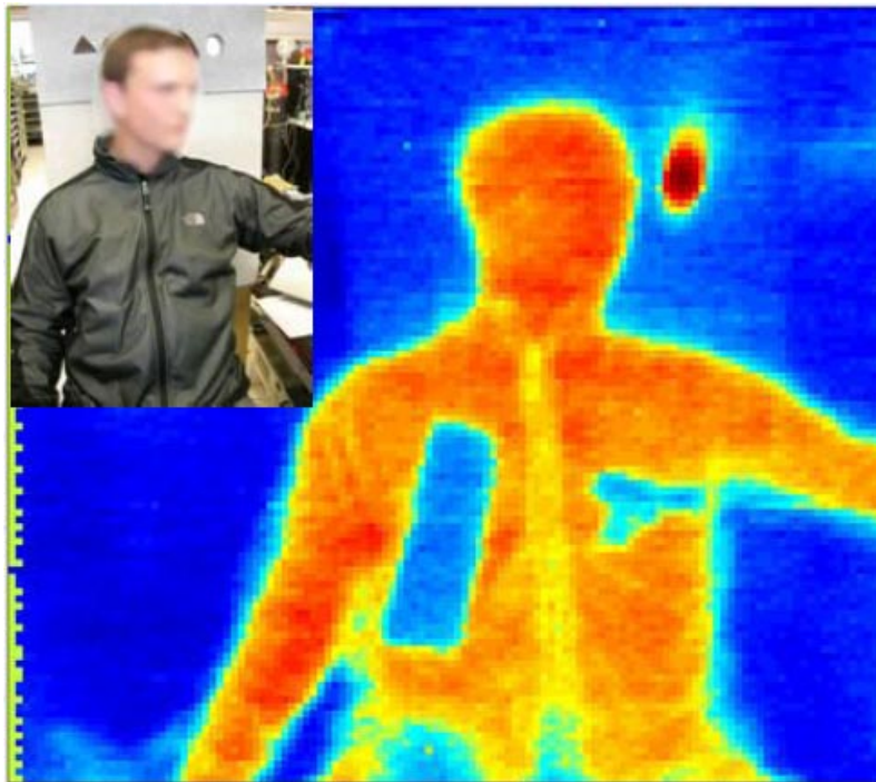
Figure 1.3: An image taken of a man (inset) carrying a gun. A single pixel HEB mixer was used to create the image [8].
