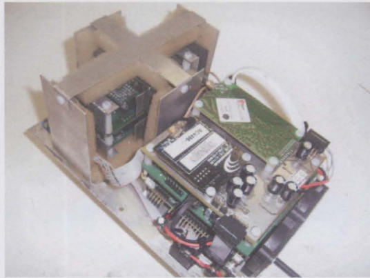
Figure A.5: Avionics system - PC104 Stack bottom right, IMU top left
