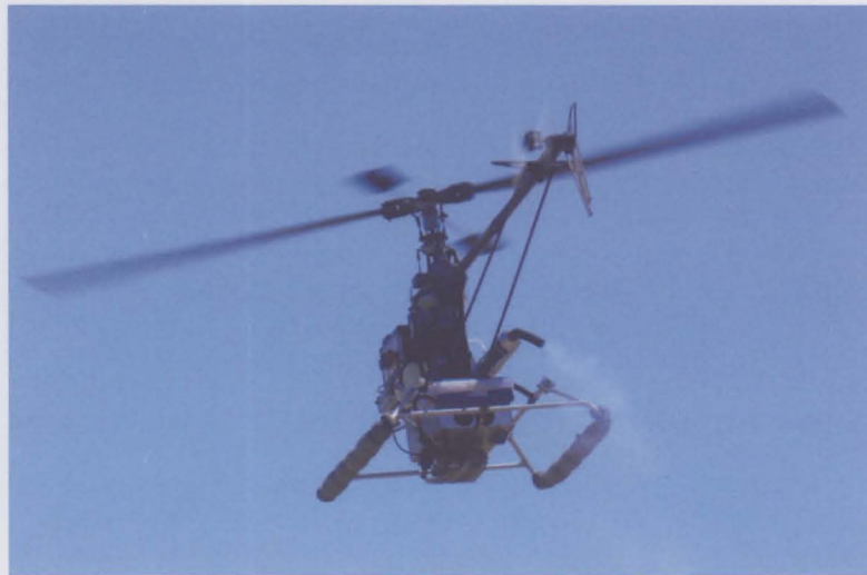
Figure A.7: X-Cell during an Autonomous hover
