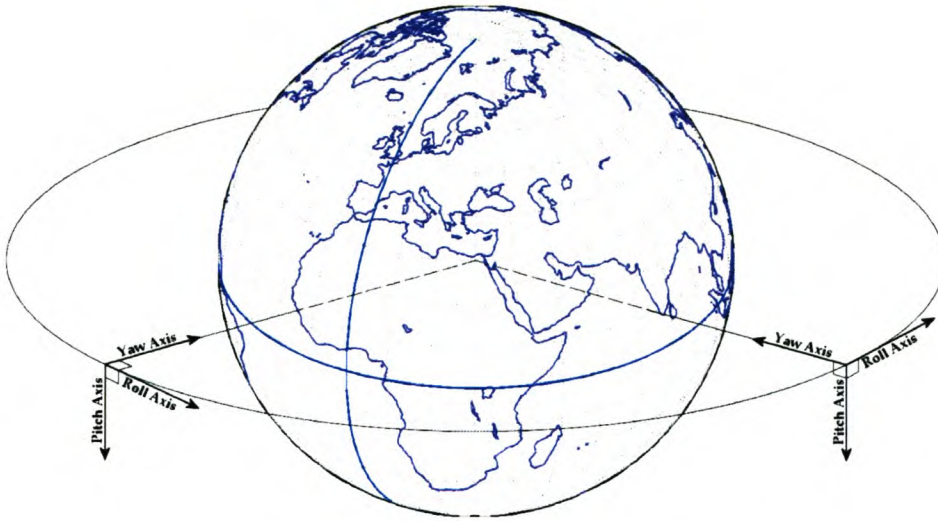
Figure A.3: Roll, Pitch and Yaw RPY Coordinates
