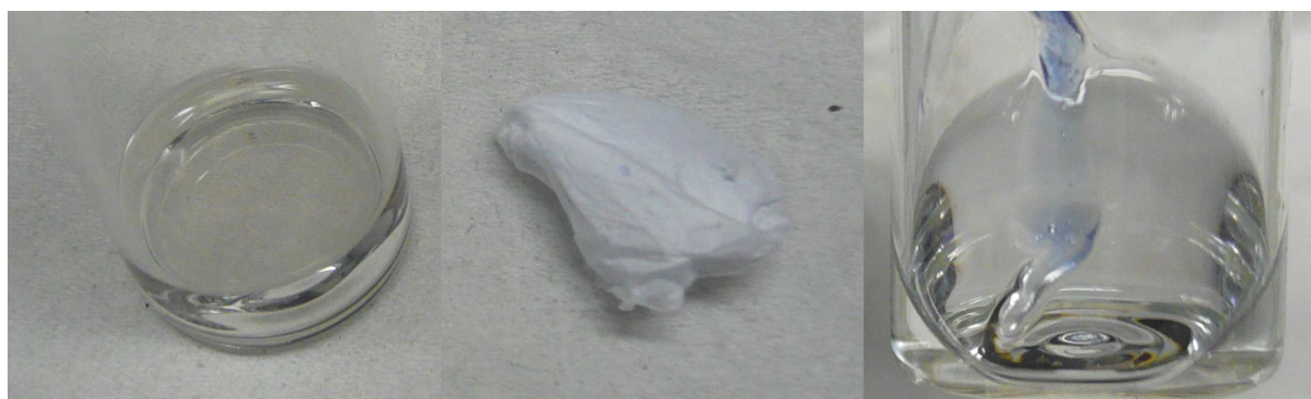
Figure 4.6 Core-shell fibres with thermochromic dye composite as core material (CA shell), before and after immersion in DCM.
