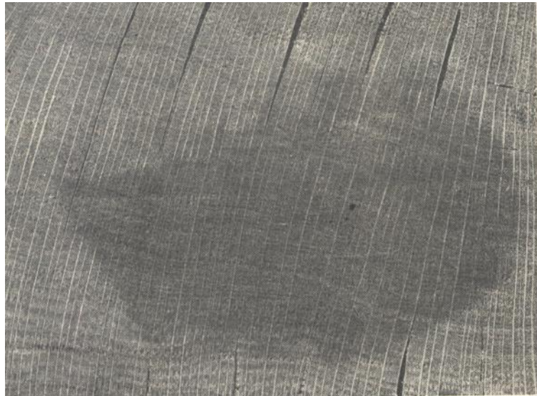
Figure 2.1b: Cross-section of an oak timber showing how surface checks follow rays (Koehler and Thelen, 1926)
