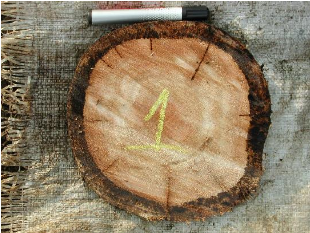
Figure 3.11: Deep surface checks in a treated Eucalyptus pole with no creosote penetration in the heartwood (Wessels et al. , 2004)
