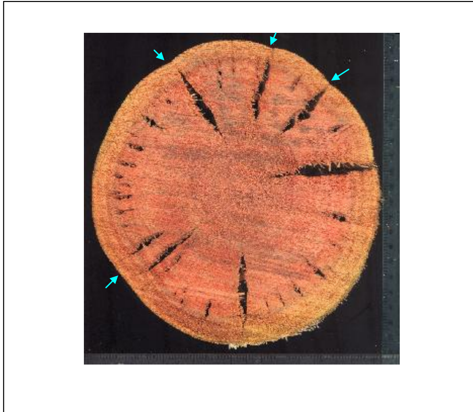
Figure 3.3 Corrugations (grooves) indicated with arrows on the outer surface of the disc at TGL
