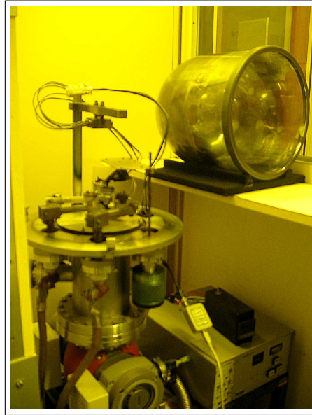
Figure 5.13: Thermal evaporation unit
