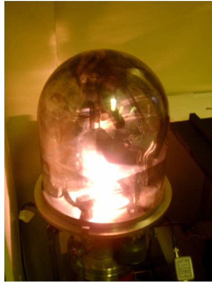
Figure 5.15: Thermal evaporation unit during annealing process
