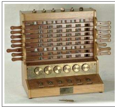
Figure 2.2: Schickardt's mechanical calculator [4]
