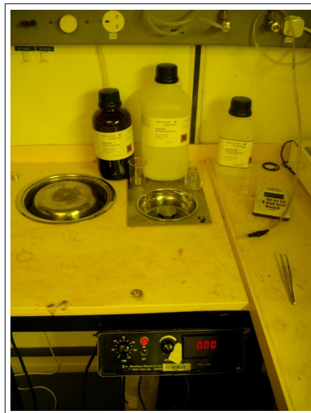
Figure 5.3: Photoresist spinner and associated chemicals
