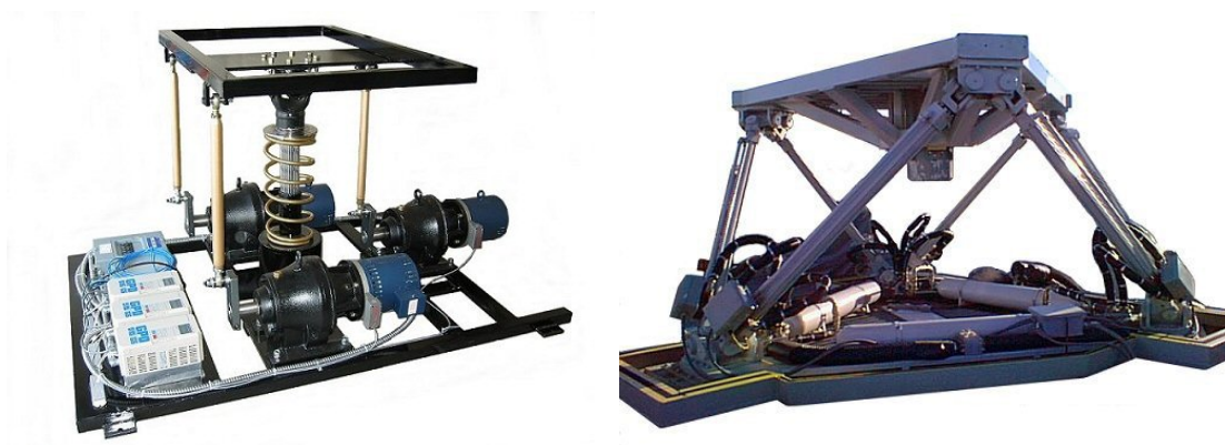
Figure 1.3 – 3-DOF and 6-DOF Motion Simulation Platform [25]
