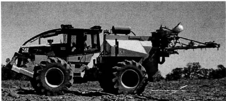
Figure 5. Second generation WS sprayer for pre-plant application of herbicide and fertilizers.
