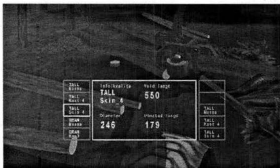
Fig. 10. Head up display with assortments according to the bucking computer.
