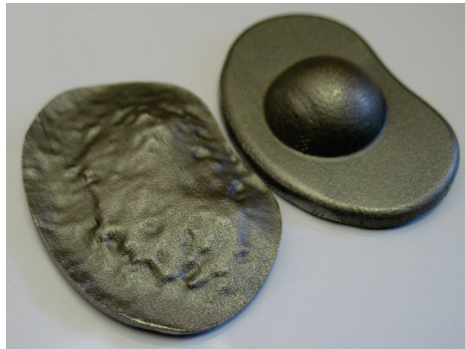
Figure 3: Rapid Manufactured patient-specific Ti_6Al_4V intervertebral disc implant
