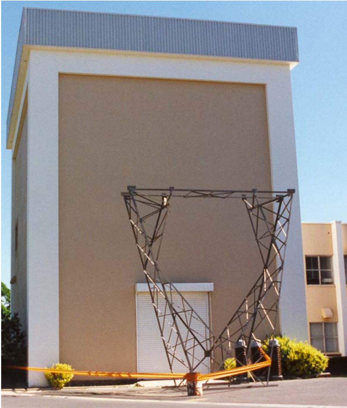
Figure B.1: 275kV tower window set up outside the High Voltage Laboratory
