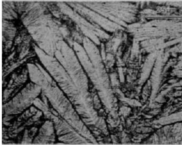
Figure 2. 12: Reflection optical micrograph of lamellae in iPP crystallized at 200 MPa and an isothermal crystallization temperature of 203°C. Lamellae are arranged in the form of feathers. The sample was etched with permanganate potassium for 30 minutes [31].
