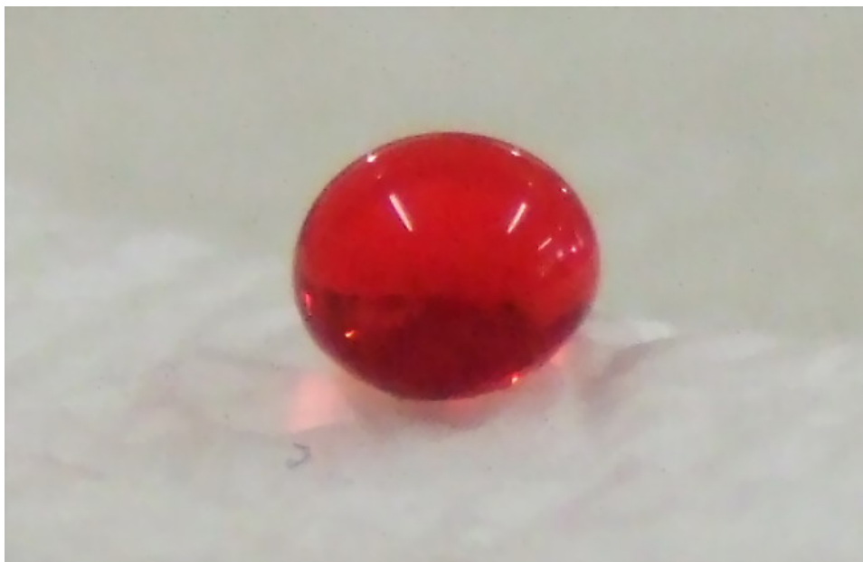
Figure A.1 Water droplet illustrating the superhydrophobicity of a PMMA-g-PDMS surface
