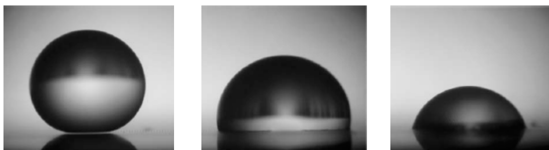
Figure 2.3 Example of different contact angles ranging from superhydrophobic to hydrophilic 19 .
