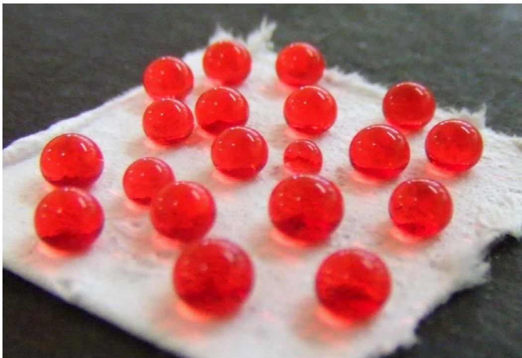
Figure A.3 Multiple water droplets illustrating the superhydrophobicity of a PMMA-g-PDMS surface.
