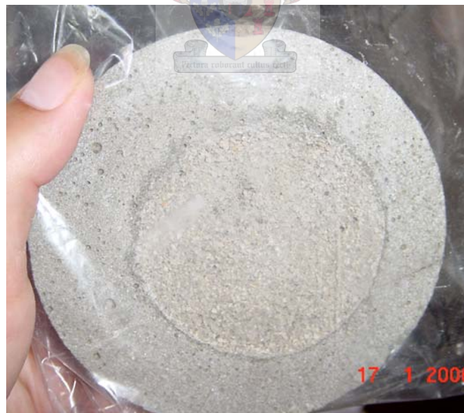
Figure 6.1.4: Minor surface decay of aggregate-added geopolymer sample (N22). Mortar samples showed severe cracking and aggressive surface decay.
