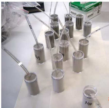
Figure 3.4.2: Embedded FlexiForce® sensors. Care was taken to place all the sensors at relatively the same location in each sample.
