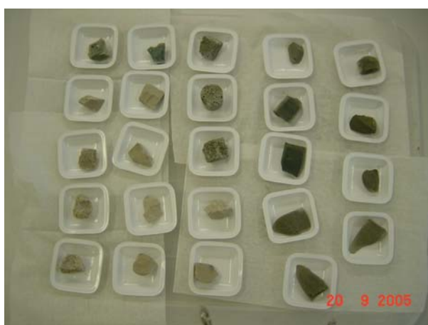
Figure 3.3.1: Sections of each geopolymer recipe were obtained and placed in a marked weighing boat. The samples were weighed before and after drying, therefore determining the total pore volume of each recipe. Here, the difference in colour of the two different fly ashes can be seen.
