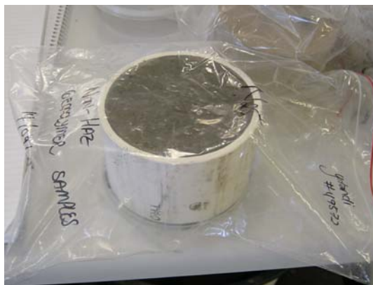
Figure 3.1.4: PVC pipe moulds with geopolymer sample. The samples are carefully marked and sealed before curing and analysis.
