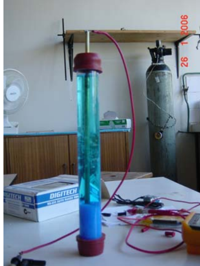
Figure 3.2.2: Copper/Copper-sulphate half cell as used to determine the extent of corrosion for embedded reinforced steel bars. The method has been commonly used by concrete researchers, but was now also introduced into geopolymer research.
