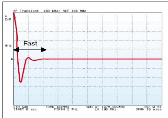
Figure 5.4 Lockup time characteristic at higher cut off frequency [17].
