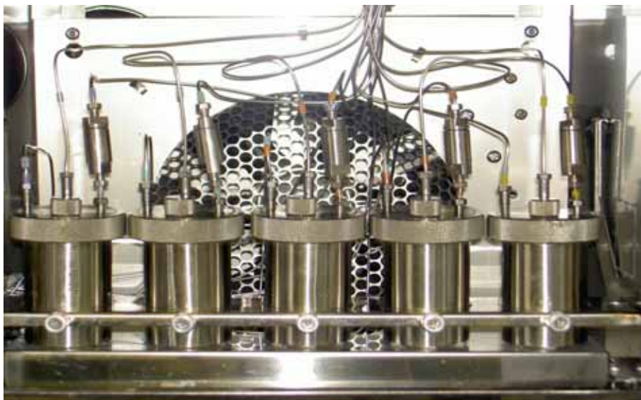
Figure 3.2 CRYSTAF setup showing stainless steel crystallization vessels inside a temperature-programmable oven.
