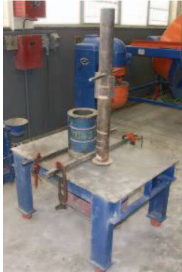
FIGURE 3-25: VIBRATORY TUBE COMPACTION SET UP
