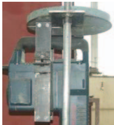
FIGURE 3-15: LEFT VIEW OF THE CONSTRUCTED MONTING HEAD FOR THE BOSCH ® HAMMER.
