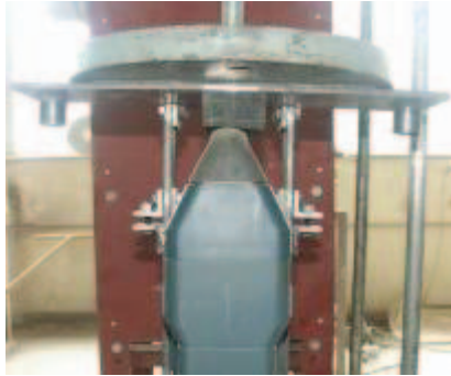
FIGURE 3-16: FRONT VIEW OF THE CONSTRUCTED MOUNTING HEAD FOR THE BOSCH® HAMMER.
