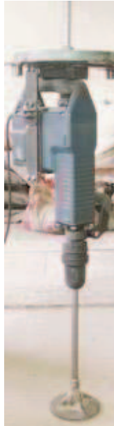
FIGURE 3-17: FULL VIEW OF THE CONSTRUCTED MOUNTING HEAD BOSCH®
