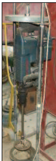
FIGURE 3-20: RAISED VIBRATORY HAMMER
