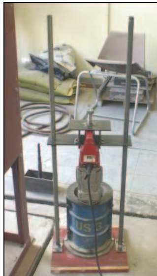
FIGURE 3-11: TOP VIEW OF THE CONSTRUCTED KANGO® MOUNTING FRAME
