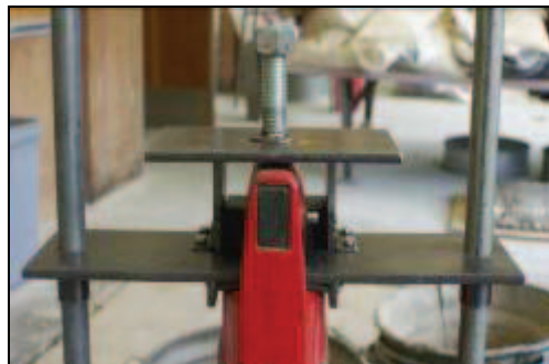
FIGURE 3-13: FRONT VIEW OF THE CONSTRUCTED KANGO® MOUNTING FRAME
