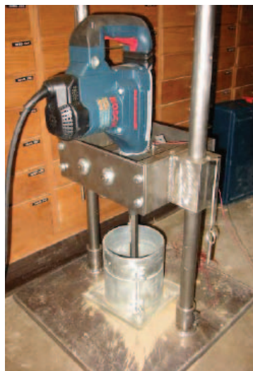
FIGURE 2-7: MOUNTING FRAME FOR ASTM VIBRATING HAMMER COMPACTION
