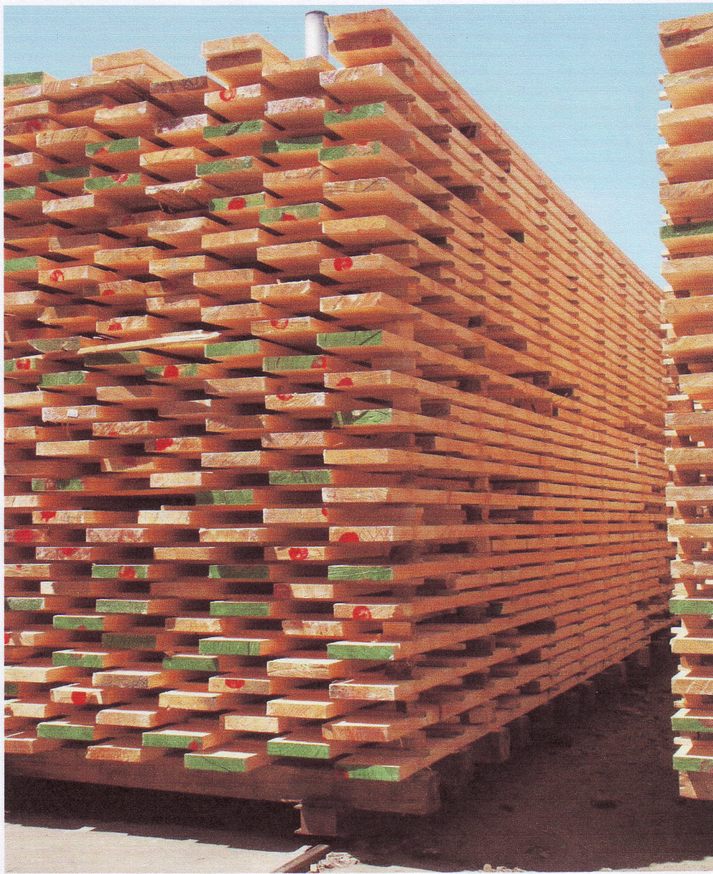
Figure 6.2: A picture of a typical cross-piled timber stack to be dried in a kiln.
