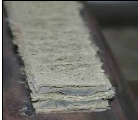
Figure 10: Close-up of fired CFM specimen, notice the irregular roving distribution.
