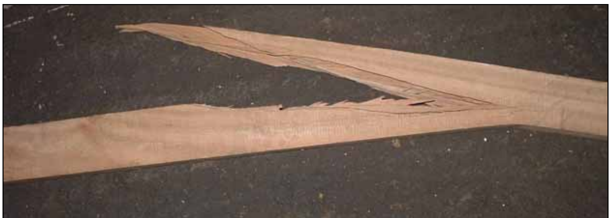
Figure 56: Failure of Saligna beam
