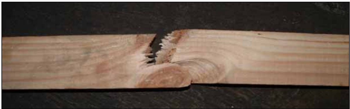
Figure 55: Failure of Pine beam
