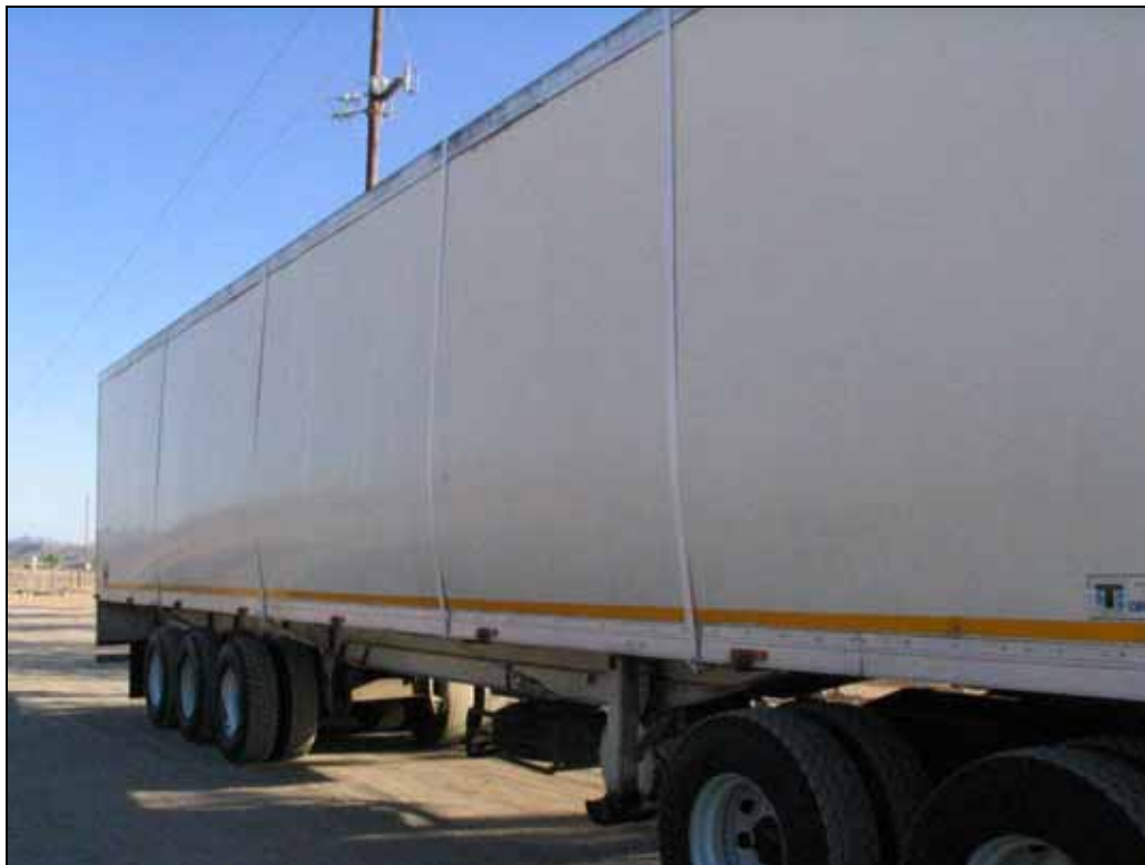
Figure 2: Close-up of failed trailer side, note the tie straps, these cause further damage.
