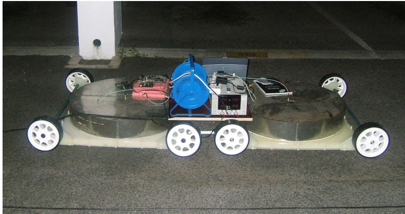
Figure 5.9: Photo of GPR measurement set-up.
