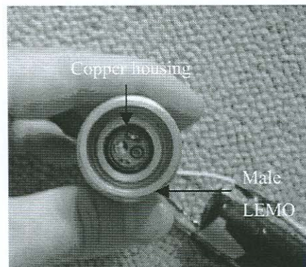
Figure 6.28 : Copper housing and LEMO connector.
