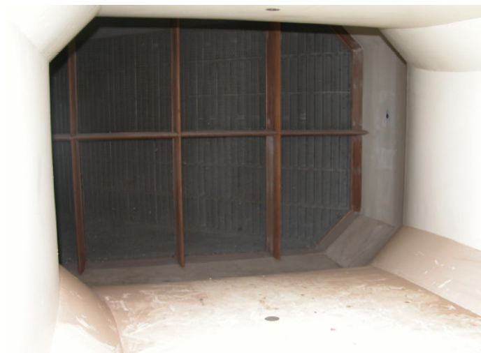
Figure C1.3: Mesh to Ensure Uniform Flow
