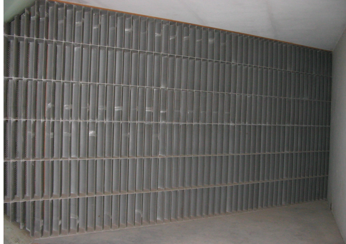
Figure C1.2: Guide Vains Turn wind flow by 90 degrees
