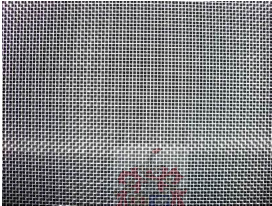
Figure A1.4: The Mesh which breaks up any Turbulence in the Wind Tunnel.
