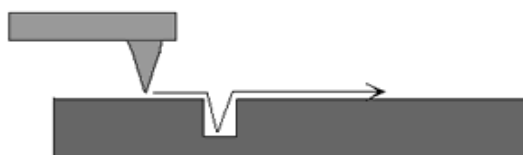
Figure 3. 4: The AFM probe scans over a hole in a surface. Because of the width of the probe, it does not reach the bottom of the hole [22].
