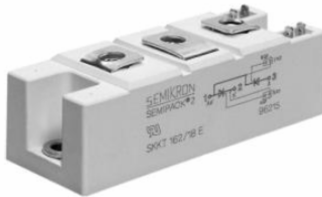
Figure 4-4: SKKT SEMIPACK 2 thyristor modules from SEMIKRON with isolated base plate
