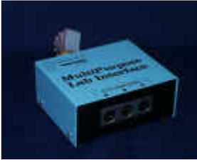
This box provides the functionality of converting the signals from the sensors to a format that can be used by the computer.
