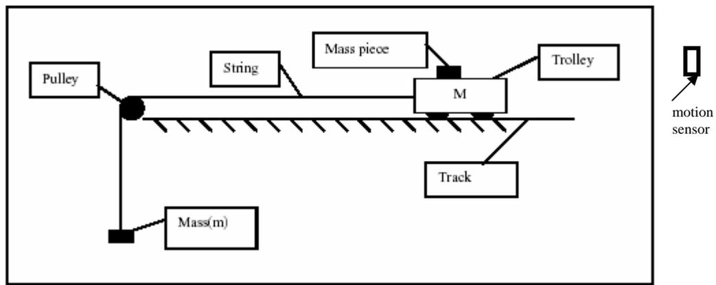
**Figure 4:** Set-up of apparatus for Activity Three.
