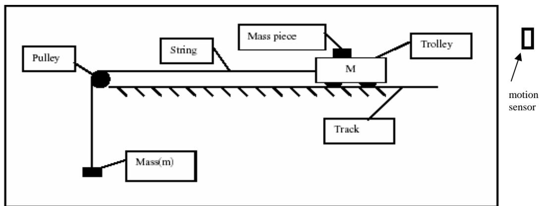
**Figure 3:** Set up of apparatus for Activity Two.
