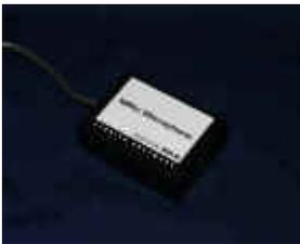
This device is capable of converting sound into an electrical signal so that it can be used by a computer for calculations.
