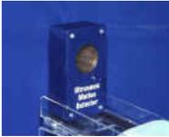
A device that measures the distance to the closest object. This is accomplished by emitting pulses and measuring the time for these pulses to be reflected.
