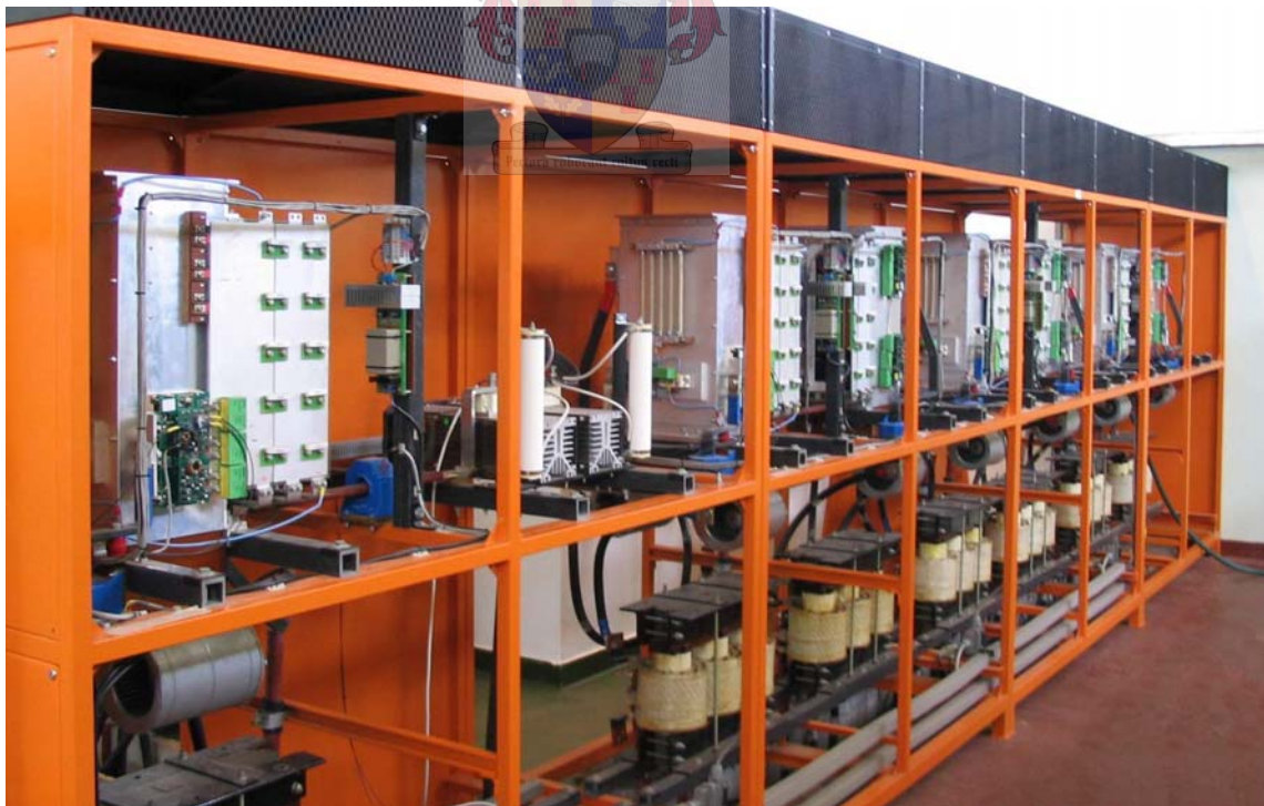
Figure 2.13 The full seven level series-stacked system
