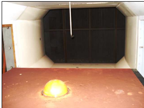
Figure 2.3: Wind tunnel intake section without additional turbulence grid
