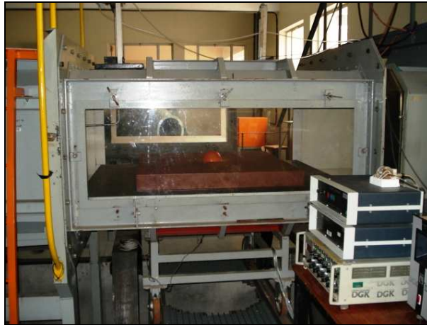
Figure 2.2: Interchangeable test section with plant model
