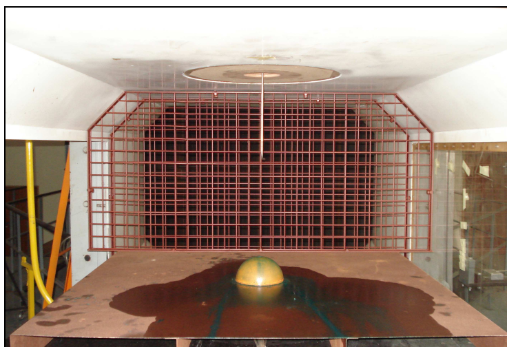
Figure 2.5: Wind tunnel inlet section with additional turbulence grid
