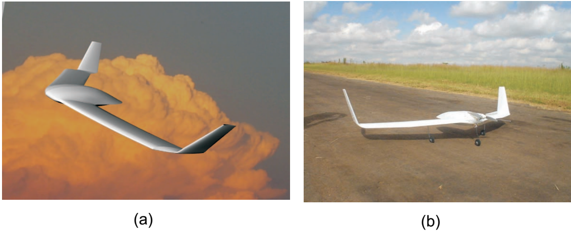
Figure 1.1: (a) Sekwa CAD model. (b) Constructed Sekwa UAV.
