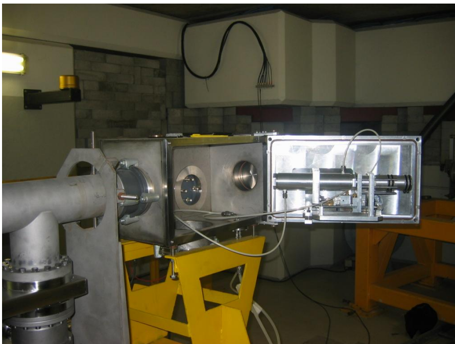
Fig. 5.9: The LiCl target holder mounted on the door of the RERAME 55 irradiation chamber. The beamline is connected onto the chamber from the left side.
