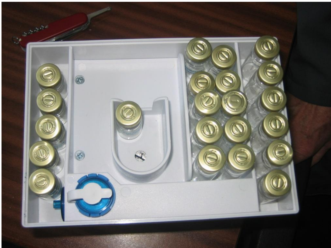
Fig. 8.3: The aerial view of the generator showing a tray carrying sterile vials.
