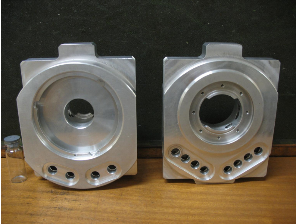
Fig. 2.5: Elephant (LEFT) and VBTS (RIGHT) target holders, with beam entrance windows and beam stops removed. The 20 mL serum vial on the left is for scaling purposes.
