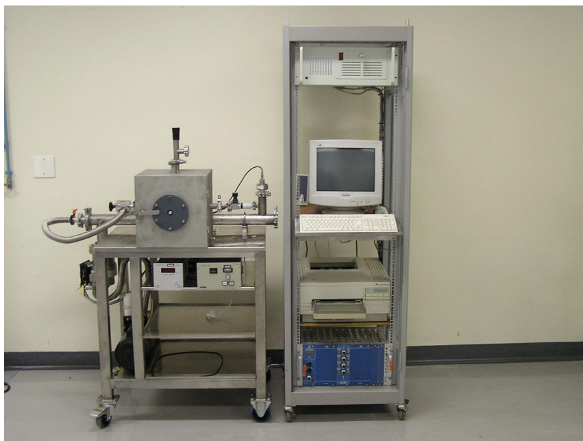
Fig. 9.6: The vacuum chamber assembly used to expose the solid state nuclear track detectors (SSNTD) to the radioactive emissions from a ^{227}\text{Pa} source (LEFT). Also shown is the multi-channel analyzer system used to acquire the \alpha -particle spectra (RIGHT).
