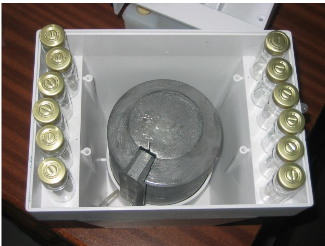
Fig. 8.4: The tray cover removed to show the shielded generator with protruding needle.
