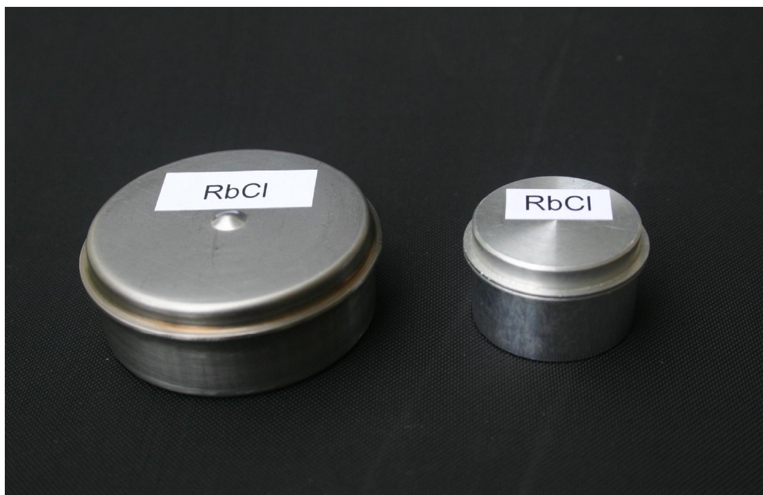
Fig. 4.4: Encapsulated RbCl targets for ^{82}\text{Sr} production. Both targets have nominally the same thickness but different diameters (outer diameters of 23 and 40 mm respectively). RIGHT: These capsules, made of aluminium, were used for many years at iThemba LABS to irradiate RbCl with a 66 MeV proton beam, up to a maximum beam current of 100 \mu\text{A} . LEFT: The new VBTS targets utilize stainless steel capsules, which are irradiated with a 66 MeV beam of nominally 250 \mu\text{A} . The increased surface area is necessary to effectively dissipate the increased heat load generated by the beam (see text).
