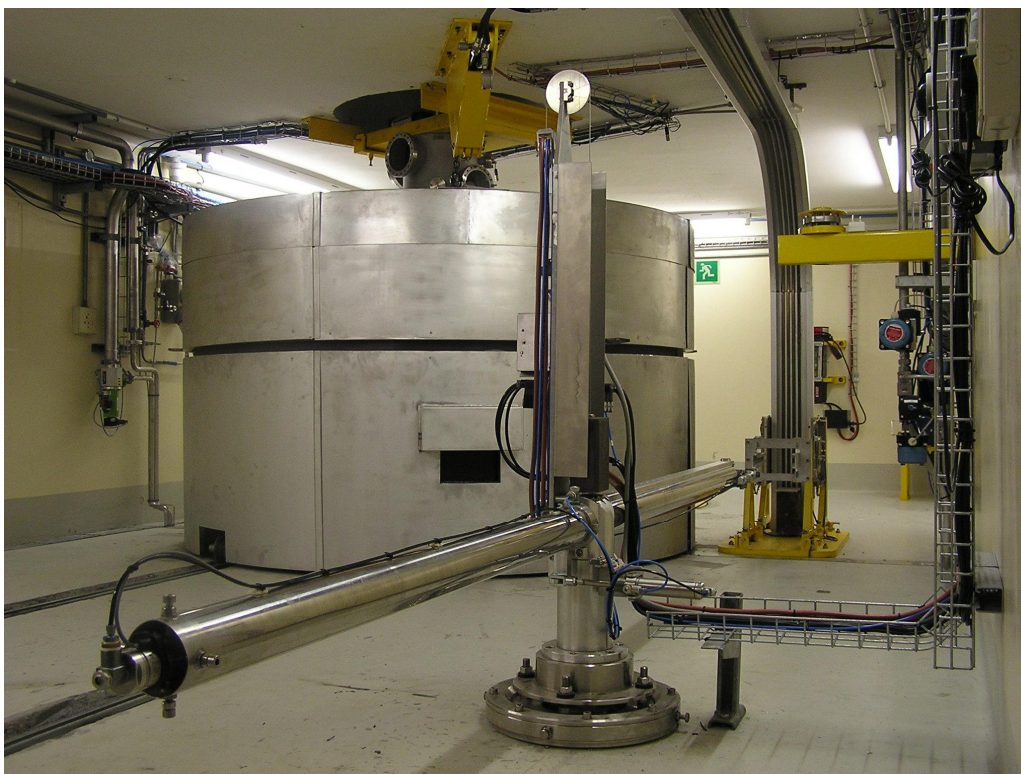
Fig. 2.3: An overall view of the VBTS 4 , a bombardment station for the irradiation of batch targets utilizing a vertical proton beam. The station is shown with the radiation attenuation shield closed. The remotely-controlled pneumatic robot arm which facilitates target transfers is shown in the foreground, while the electrified rail for target transport can be seen in the background. Note the beam diagnostics chamber on top of the target station.
