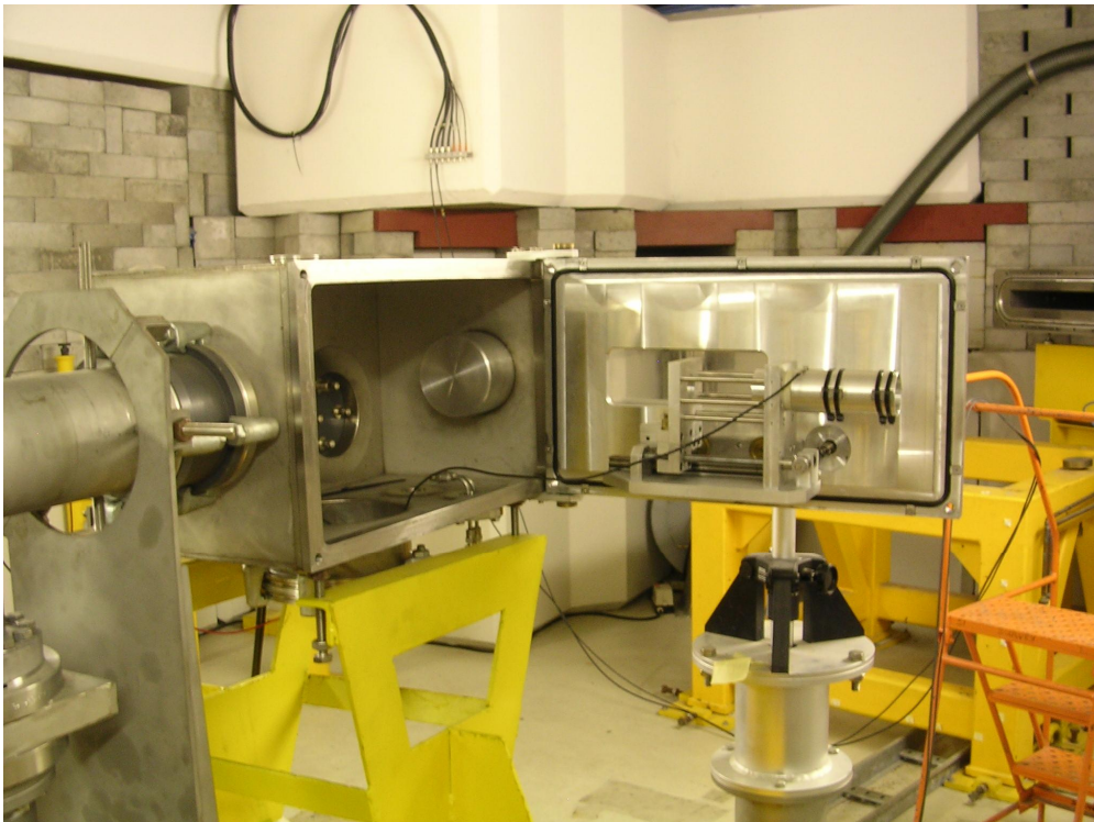
Fig. 2.6: The modified RERAME activation chamber at iThemba LABS, shown with the door in an open position. Targets or foil stacks are mounted on the door, in a vice moving on rails, in order to ensure good positional accuracy. The beam is incident from the left.
