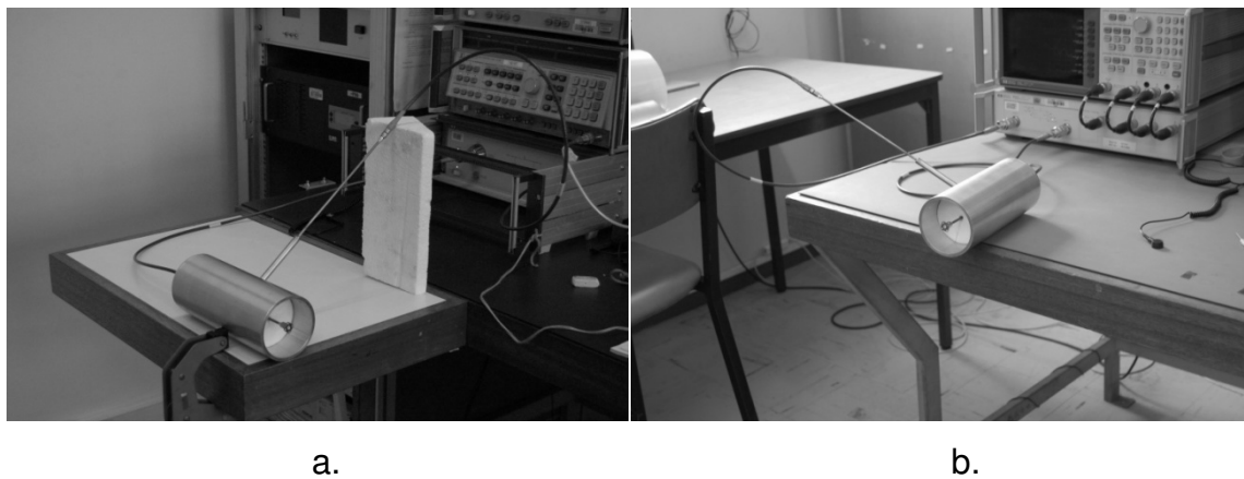
Figure 6-10: The physical setup for the two VNAs used a. Agilent 8510 and b. Agilent 8753. In both setups the same highly phase stable cables from Suhner were used
