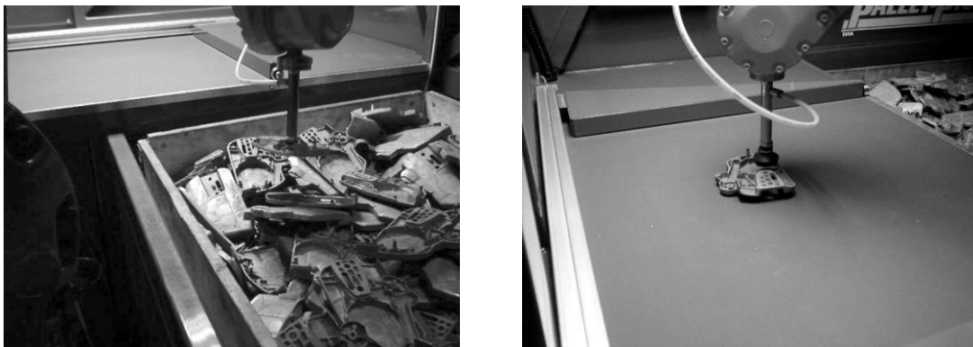
Figure 5 PalletPicker-3D bin picking with suction cup gripper [left] and re-orientation operation using flat surface [right] (Saldner 2003)
