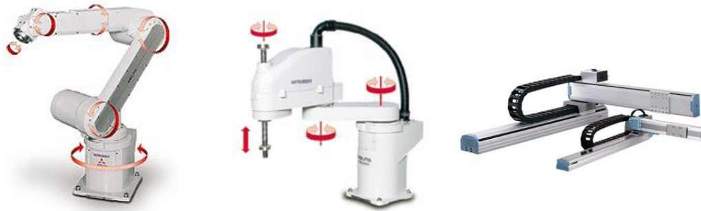
Figure 8 Three common classes of industrial robots: Articulated, SCARA and gantry (EXPO21XX 2008; EXPO21XX 2007) – from left to right
