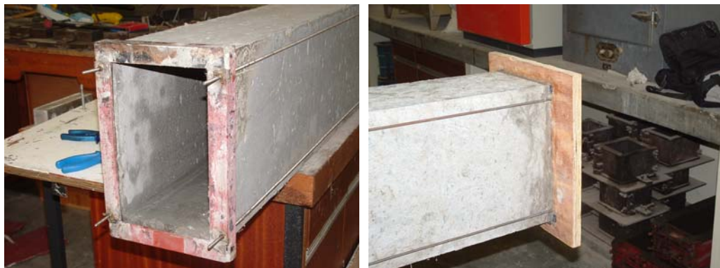
Figure 7.9 Tension rods and board to contain fresh concrete
