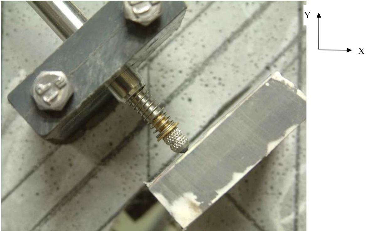
Figure 5.9 LVDT fixed on the surface of specimen
