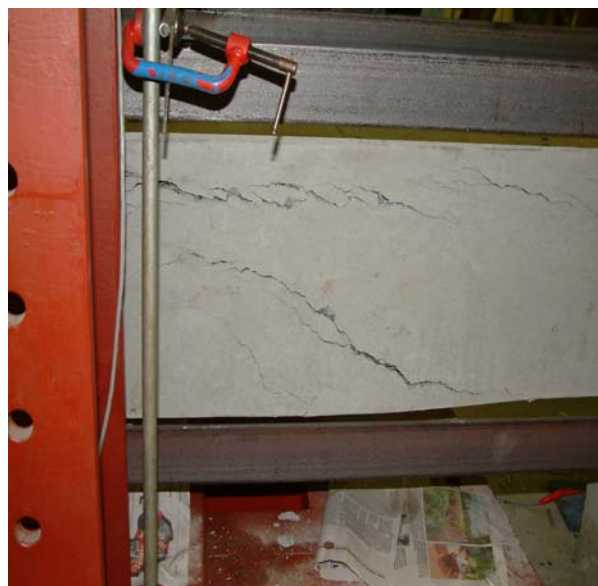
Figure 7.12 Shear failure pattern of R/C column
