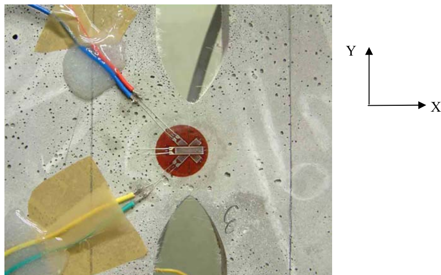
Figure 5.8 The strain gauges stuck onto the surface of specimen
