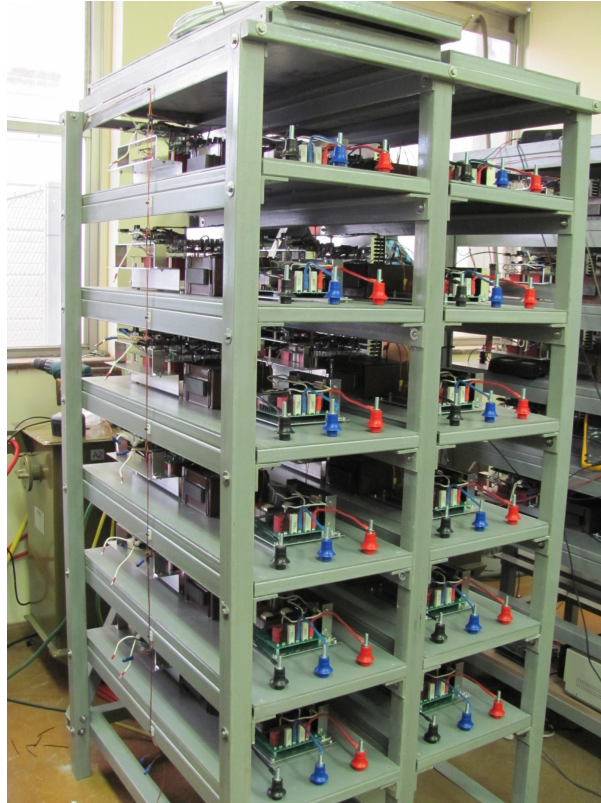
Figure 1.3: Twelve-cell stack of the 6.6 kV SST.
