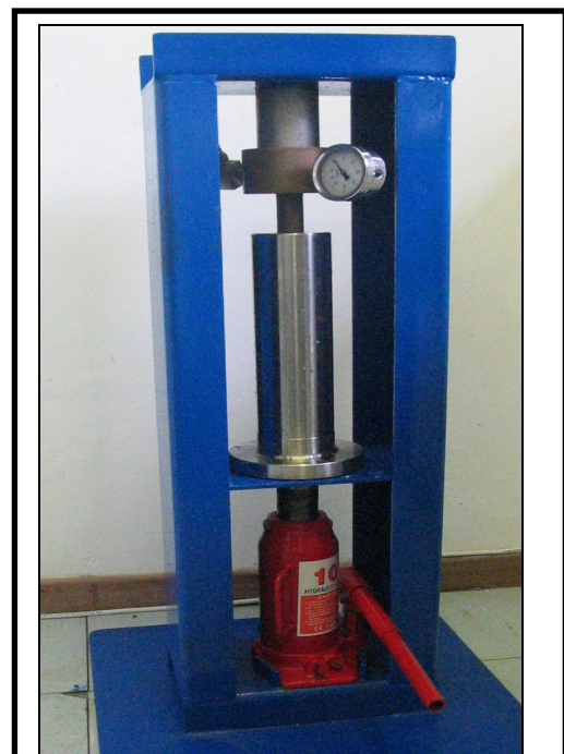
Figure 1-1 The pressure induction apparatus
