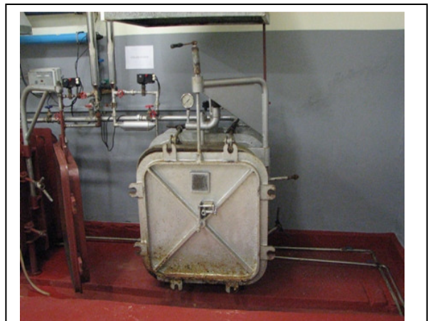
Figure 5-5 Cans placed in a steam cooker for a heat retort.
