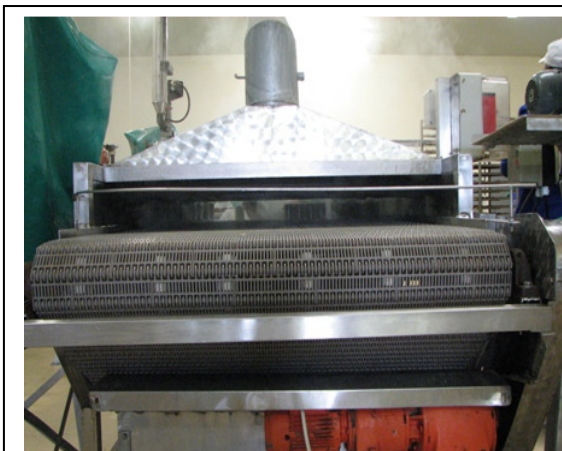
Figure 5-4 Sealed cans are sterilized in a steam machine.
