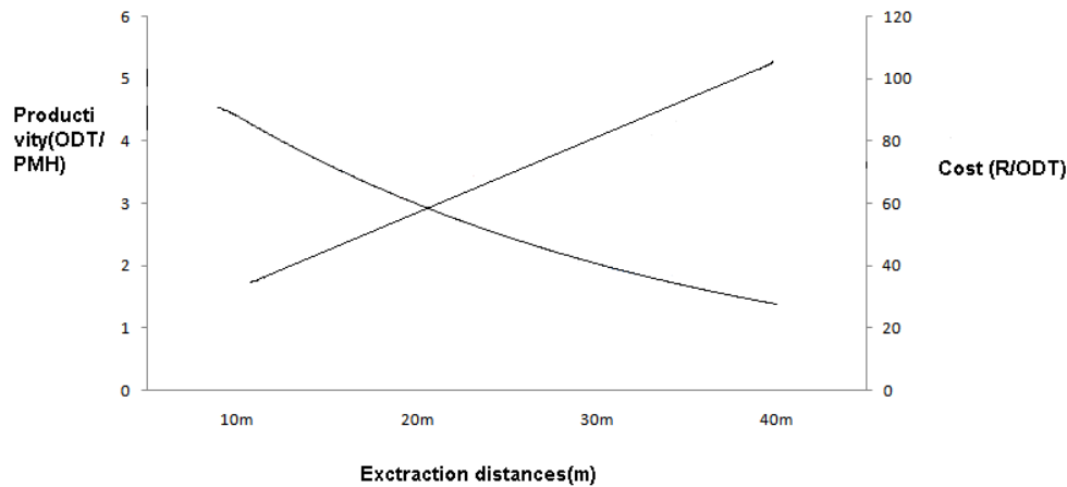
Figure 48: Interaction between cost and productivity based on various extraction distances of the three-wheeled loader (falling curve represents productivity, and rising curve the costs involved).
