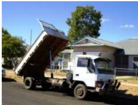
Figure 16: Truck with carrier bin without raised load body sides.
