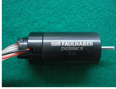
Figure 4.22: Faulhaber 2342CR brushed DC motor - EFU 7
