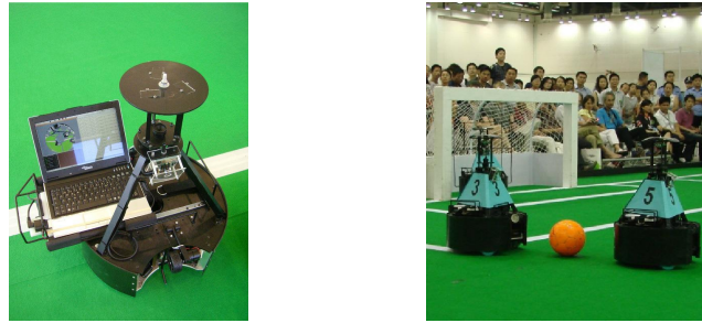
(a) Medium Size League (MSL) robot with onboard laptop (b) Medium Size League (MSL) robots and soccer ball
