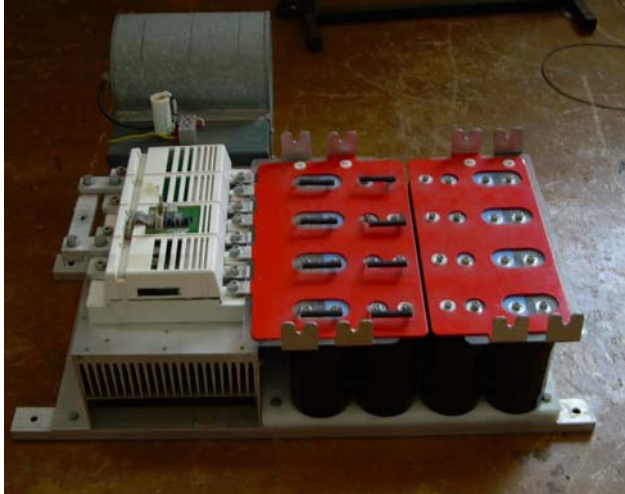
Fig E.6: IGBT phase arm unit with bus capacitors and cooling.
