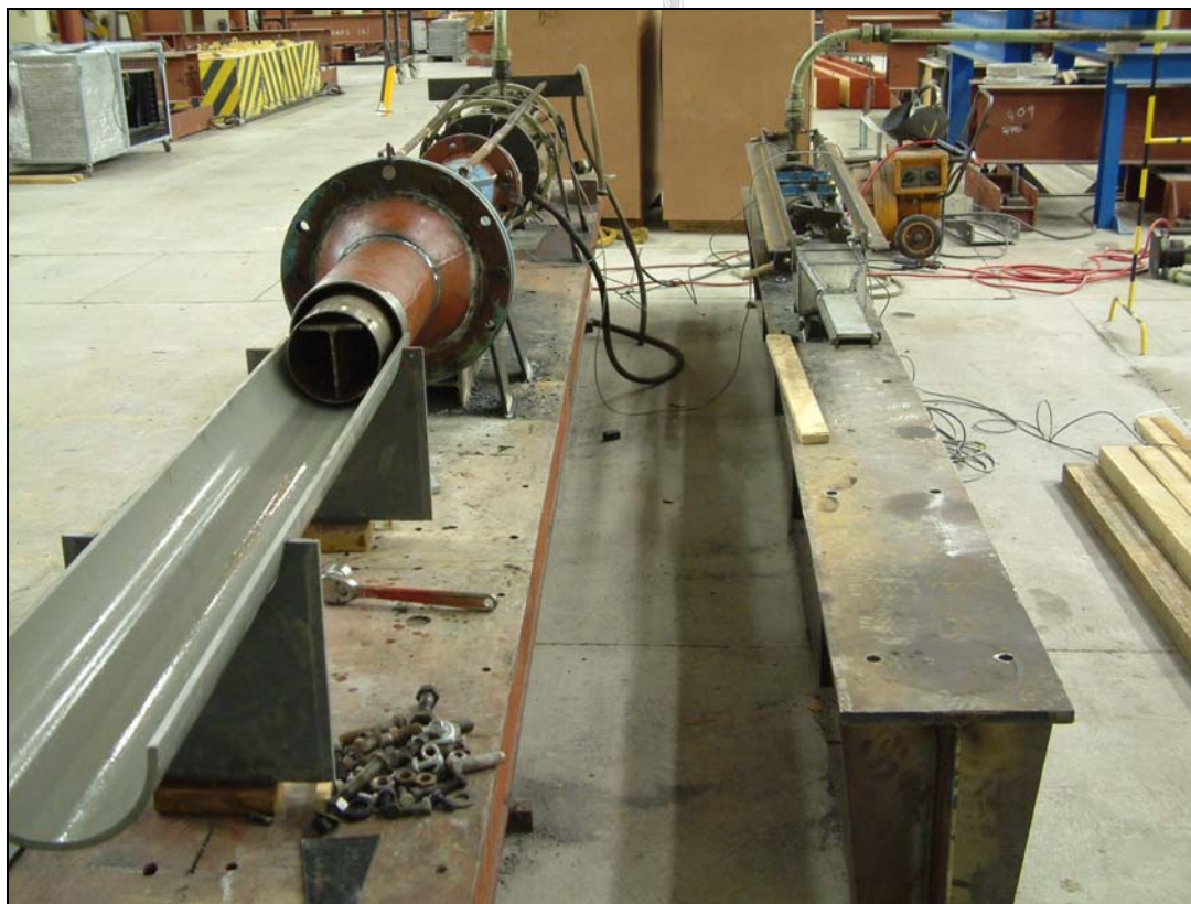
Figure 36: The pipe piston extruder (above left) and the plate piston extruder (above right)
