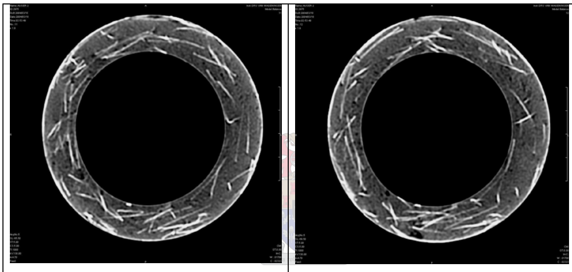
Figure 67: CT scan images of auger extruded steel fibre reinforced ECC pipe
