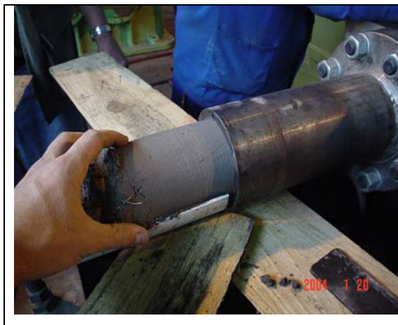
Figure 22: Auger extrusion of a pipe
