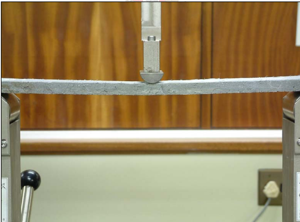
Figure 32: Three point bending setup for flexural tests
