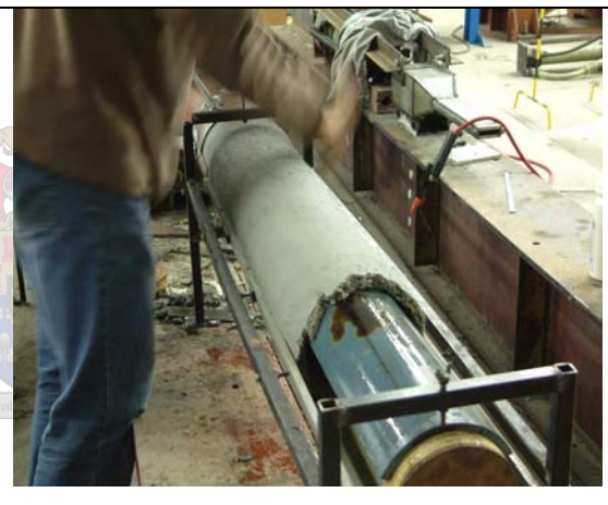
Figure 23: Piston extrusion of a pipe
