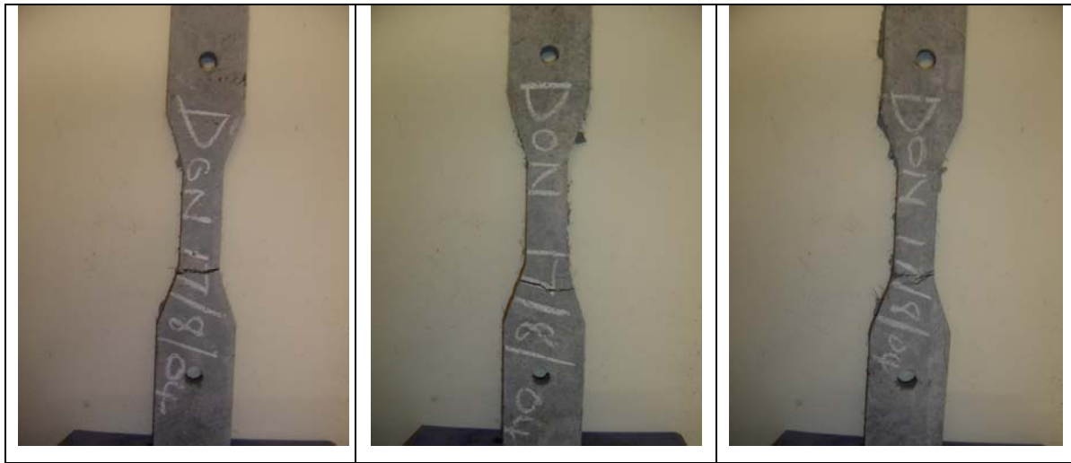
Figure 46: Tensile test specimens with single matrix cracking domination
