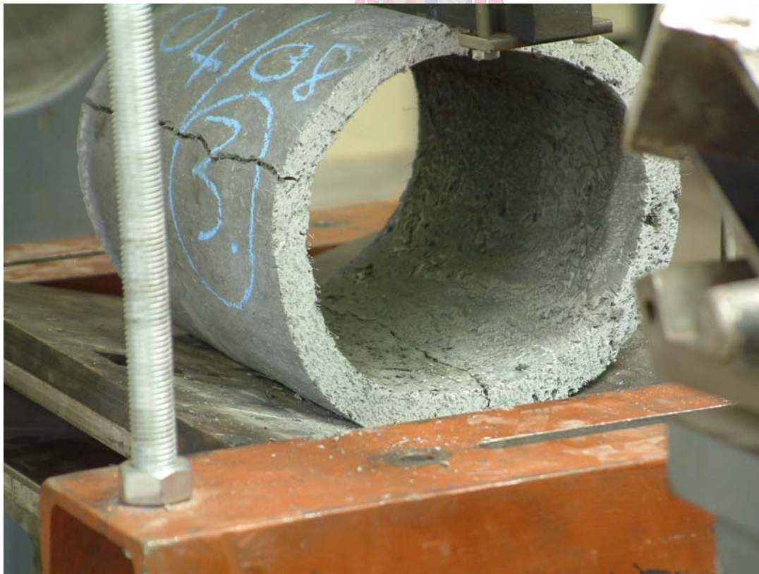
Figure 55: Anisotropic behaviour of piston extruded pipes in crushing tests
