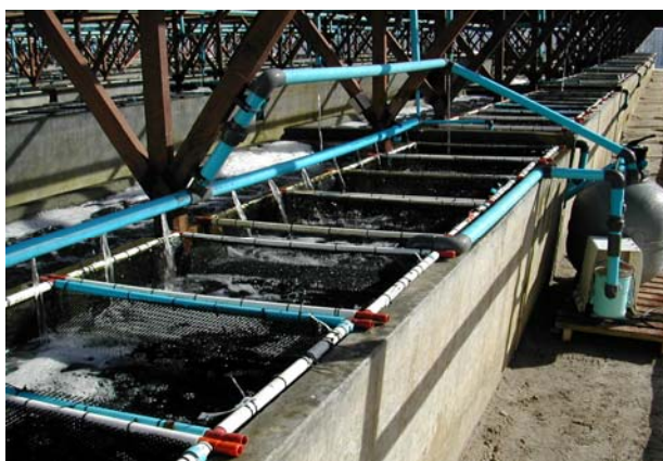
Figure 2.1 The layout of tanks and baskets in Experiment 1 to investigate the effect of water filtration on sabellid infection in abalone, H. midae .
