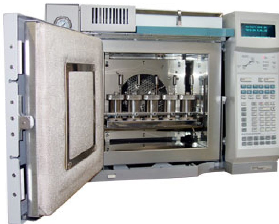
Figure 2: A typical CRYSTAF instrument showing the position of the five reactors inside the temperature-controlled oven.
