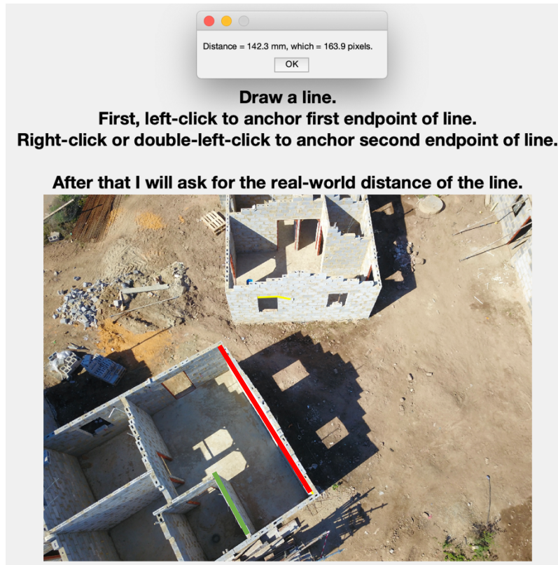
Figure 30. Length Being Measured on MATLAB Software (Green Line)
