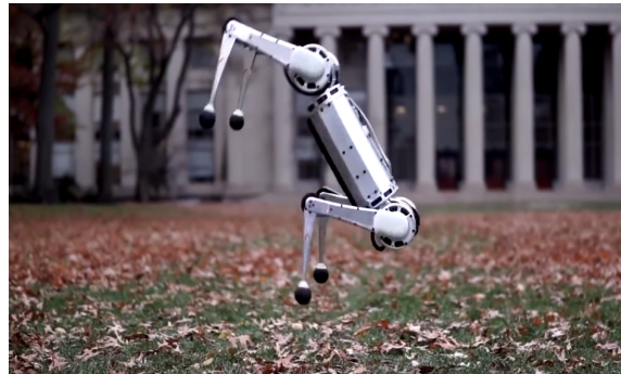
(b) The MIT Mini Cheetah quadruped robot displaying its dynamic and agile capabilities during a perfect back-flip maneuver. Image from [20].
