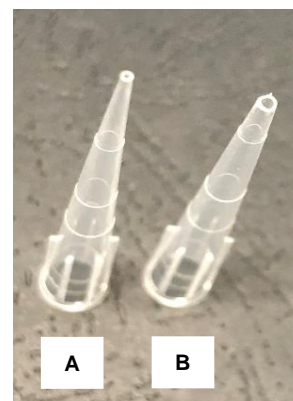
Figure 5.3 - 20-200 µL pipette tips. (A) Unaltered tip; (B) Manually altered tip.
