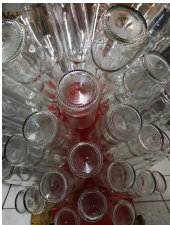
Figure 95: Draining of sulfur after sulfurization
