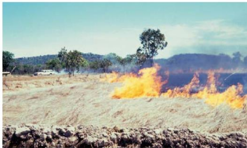
FIGURE 2.4: A typical back fire. Note flames burning from the base of the fuel bed and leaning over burnt ground. Experimental fire A011, NT, Australia, 30 July 1986. Reprinted from “Grassfires: fuel, weather and fire behaviour (2 nd ed.)”, by Cheney, P., & Sullivan, A., 2008, pp. 23, Australia: CSIRO Publishing. Copyright 2008 by CSIRO.
