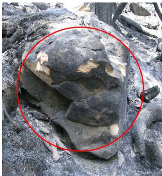
FIGURE 2.40: Example of fire-induced spalling surrounded by sooting. Reprinted from the “Guide to wildland fire origin and cause determination (2016 ed.)”, by NWCG, 2016, pp. 71, USA: National Wildlife Coordinating Group.
