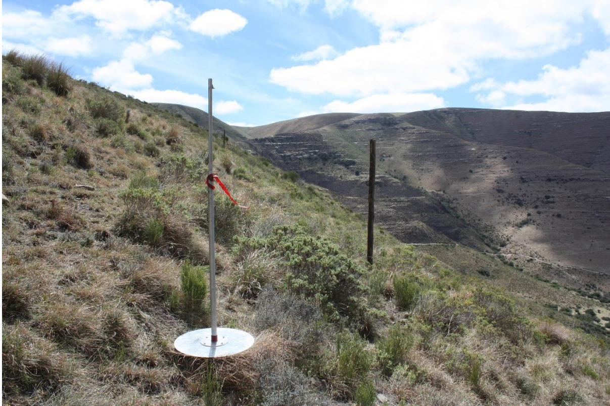
FIGURE 4.4: Photograph showing example of fence post of a known height planted at centre of 100 m 2 burn plot. Pre-planted fence posts were used for both active flame length visual observation and post-fire height of char measurements. Disc pasture meter (DPM) used for fuel load estimations is shown in foreground and to left of fence post. Prescribed burn BE3, 8 November 2019, Katberg, Eastern Cape.
