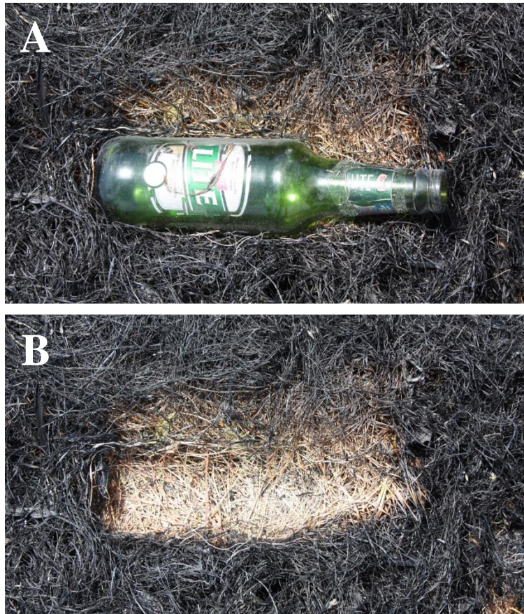
FIGURE 5.16: Example of protection fire pattern indicator, with (A) and without (B) supporting item (330 ml glass bottle). Fire passage approximately down – up. Experimental burn plot 2, Site 3. Prescribed burn DE1, Katberg, EC, South Africa, 15 October 2019.
