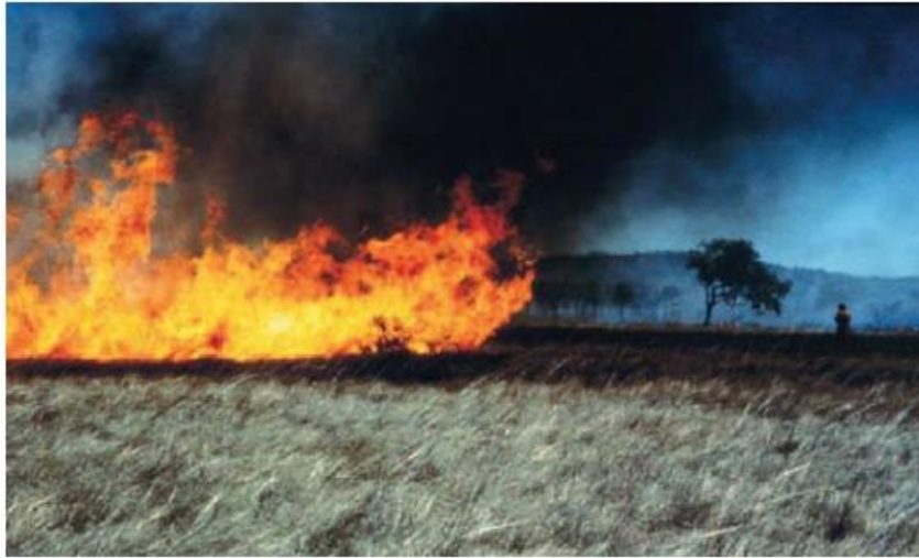
FIGURE 2.2: A typical head fire. Black smoke indicates incomplete combustion. Experimental fire A091, NT, Australia, 4 August 1986. Reprinted from “Grassfires: fuel, weather and fire behaviour (2 nd ed.)”, by Cheney, P., & Sullivan, A., 2008, pp. 22, Australia: CSIRO Publishing. Copyright 2008 by CSIRO.
