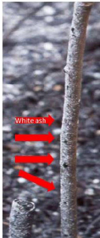
FIGURE 2.27: Example of white ash deposits blown by wind onto windward side of stem. Reprinted from the “Guide to wildland fire origin and cause determination (2016 ed.)”, by NWCG, 2016, pp. 90, USA: National Wildlife Coordinating Group.
