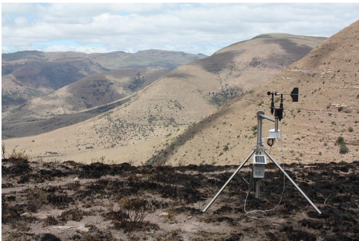
FIGURE 4.1: Photograph showing portable weather station (Campbell Scientific; R.M. Young Company) used to record wind speed & direction, ambient air temperature, and relative humidity.
