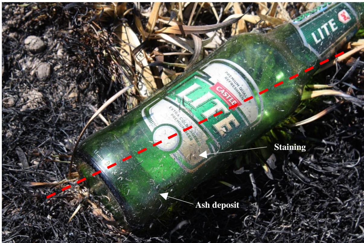
FIGURE 5.20: Example of ash deposit on stained 330 ml glass bottle. Experimental burn plot 17, site 3. Prescribed burn DE1, Katberg, EC, South Africa, 15 October 2019.
