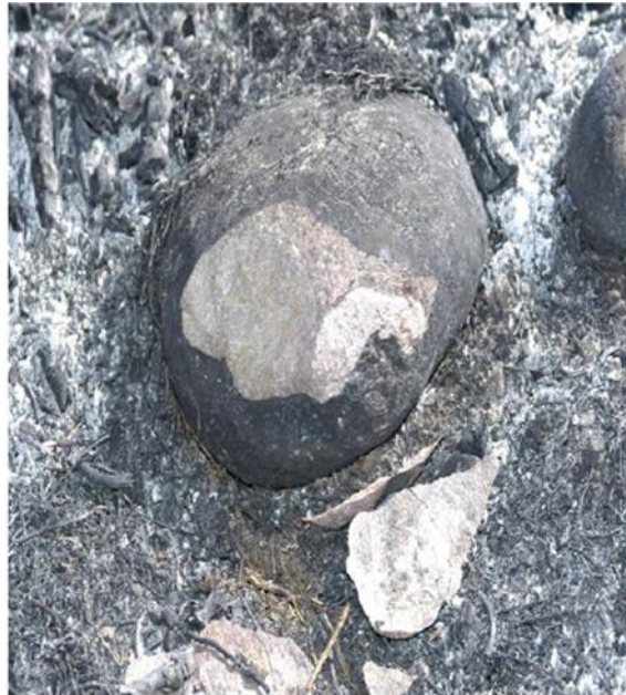
FIGURE 2.41: Example of fire-induced spalling on a rock. Fire passage bottom to top. Reprinted from the “Guide to wildland fire origin and cause determination (2016 ed.)”, by NWCG, 2016, pp. 73, USA: National Wildlife Coordinating Group.
