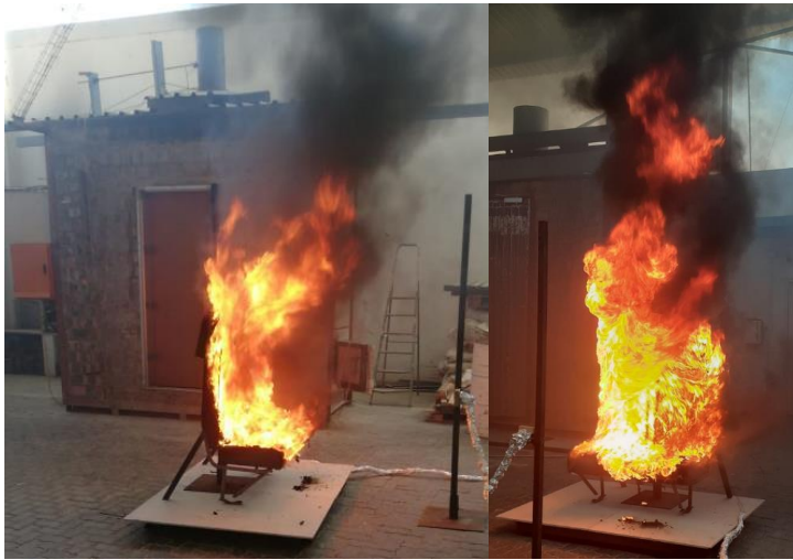
Figure 6.4: Turbulent flames leaning forward (left), fully developed stage Experiment 1 (right)
