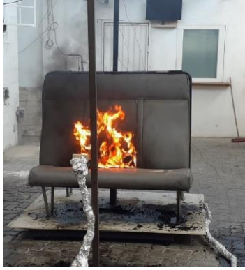
Figure 6.16: Experiment 4 ignition of seat
