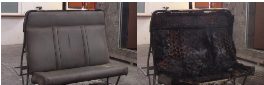
Figure 6.15: Condition of seat before and after Experiment 4
