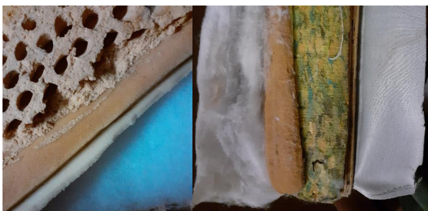
Figure 3.15: Material layers of seat back and seat bottom
