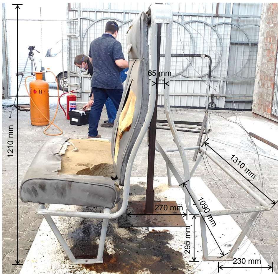
Figure 4.7: Dimensions of frame for Experiment 2, 3 and 4
