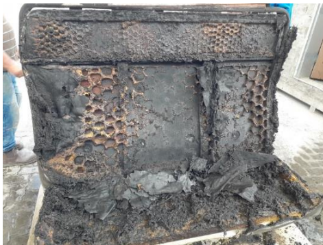
Figure 6.19: Seat after Experiment 4
