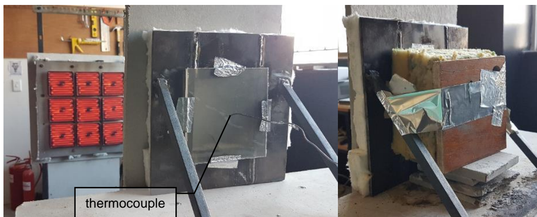
Figure 4.3: Sample positioning and thermocouple placement
