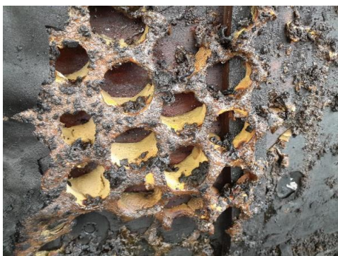
Figure 6.20: Melted foam after Experiment 4
