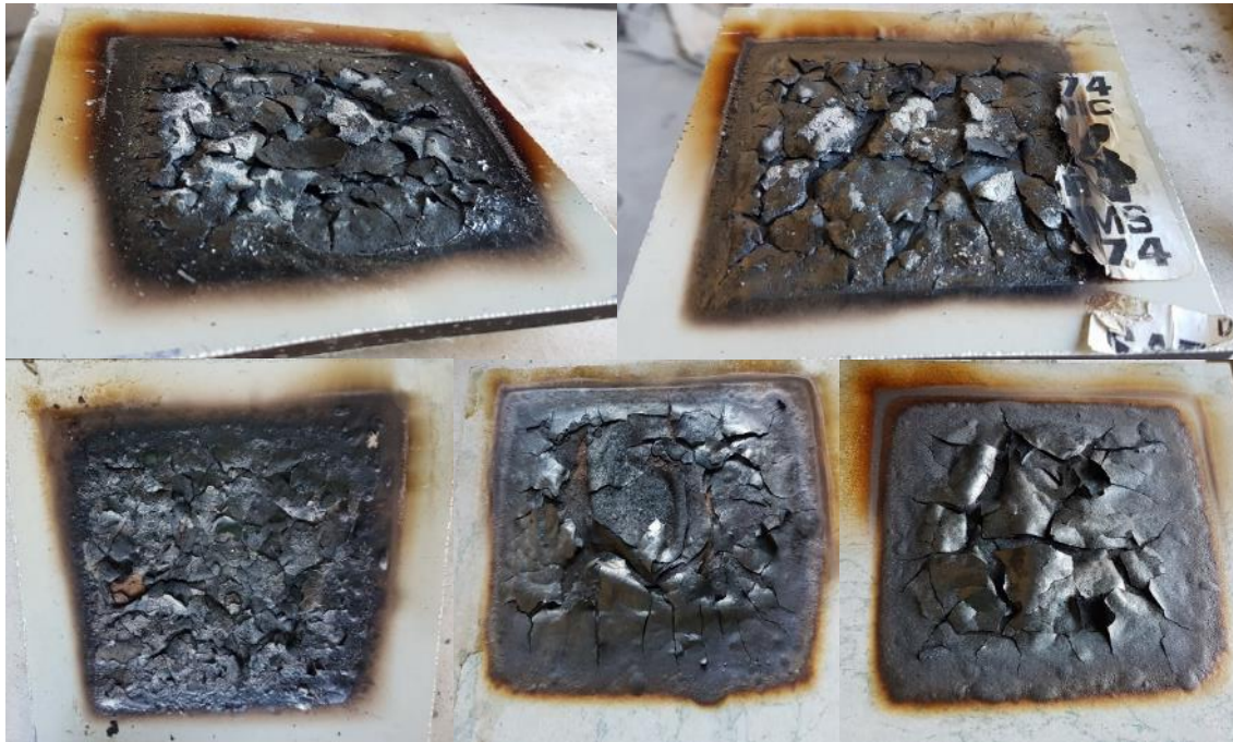
Figure 5.2: Bakelite (C_B_M and C_B_P) samples after radiant panel tests
