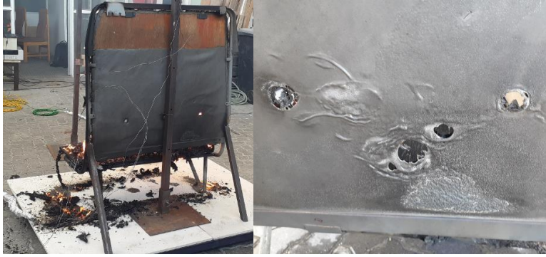
Figure 6.6: Seat back at end of Experiment 1
