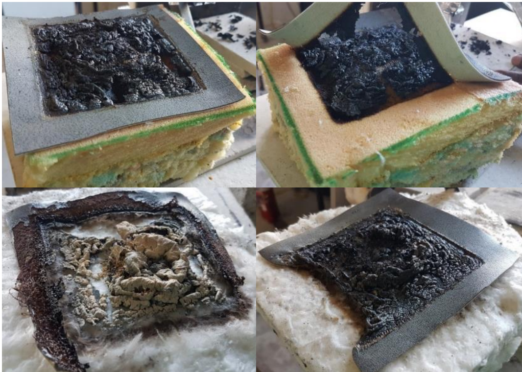
Figure 5.5: Pleather (S_PI_F) samples after radiant panel tests
