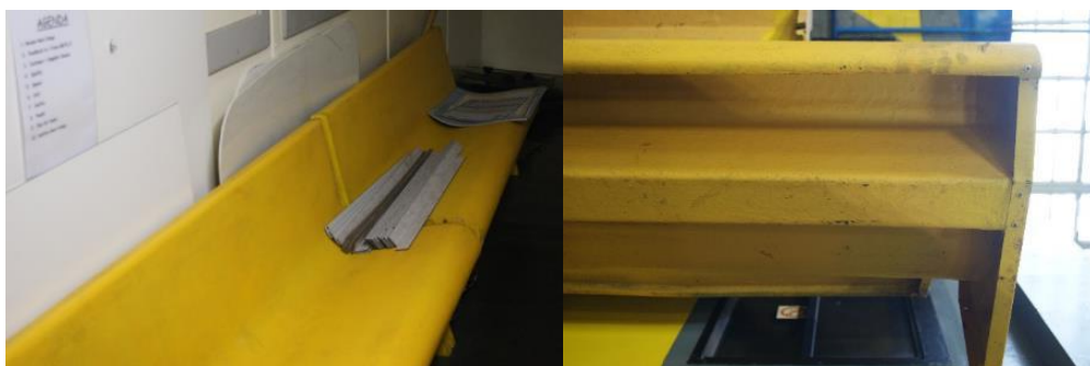
Figure 3.5: Metro fibreglass seats
