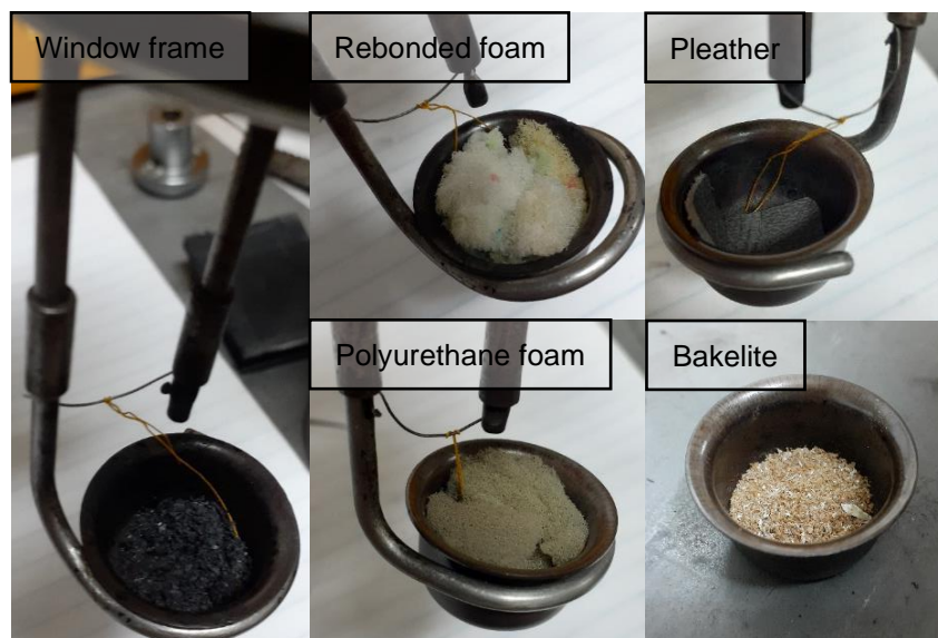
Figure 4.1: Sample preparation for bomb calorimeter testing
