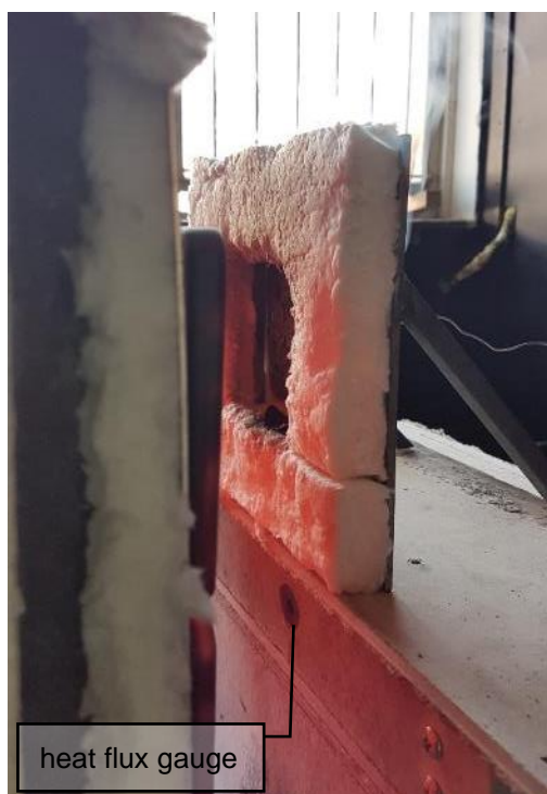
Figure 4.4: Positioning of water-cooled heat flux gauge
