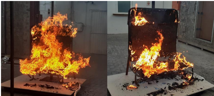
Figure 6.5: Decay stage of Experiment 1
