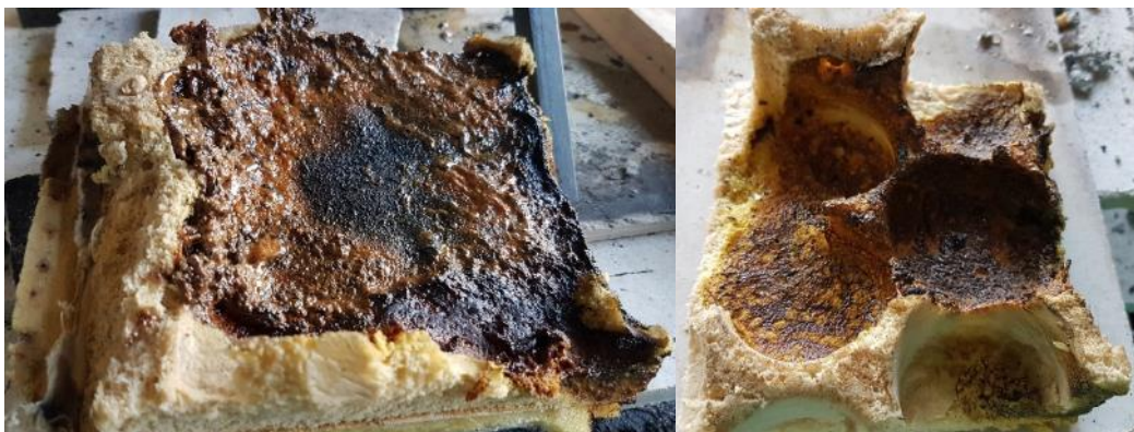
Figure 5.6: Rubbery foam (S_Ru_C) samples after radiant panel tests
