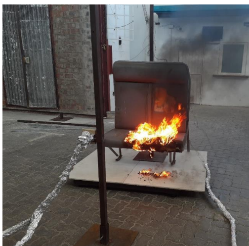
Figure 4.9: Experimental setup for full-scale seats showing the chairs soon after ignition
