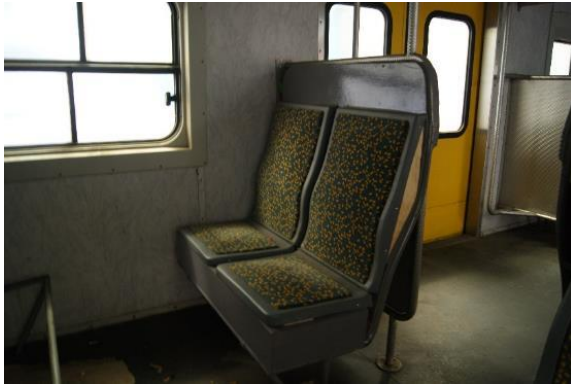
Figure 3.6: Retrofitted seat in a 5M2A carriage
