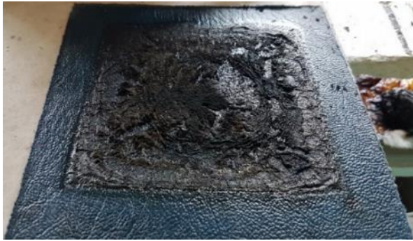
Figure 5.4: Blue pleather (S_PIPW) sample after radiant panel tests
