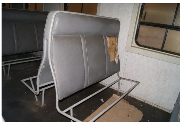
Figure 3.14: Seats in carriage at Salt River depot workshop with seat bottoms already stripped
