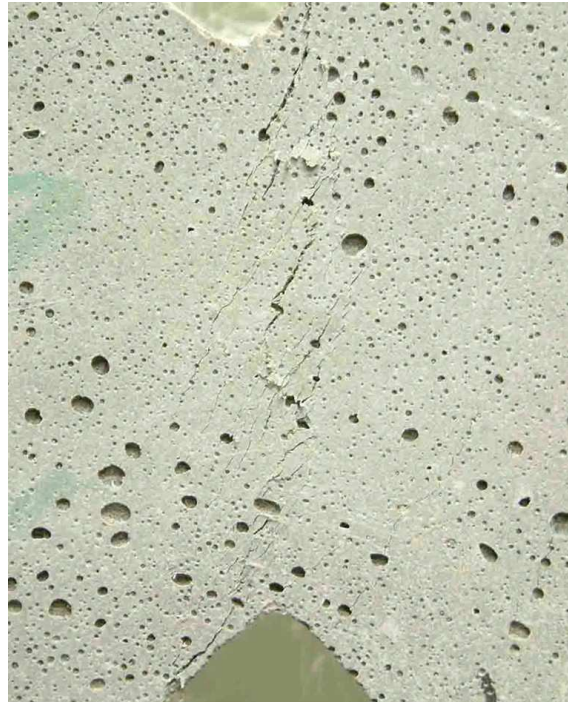
Figure 6.26 The final localising experimental crack pattern from Shang (2006).
