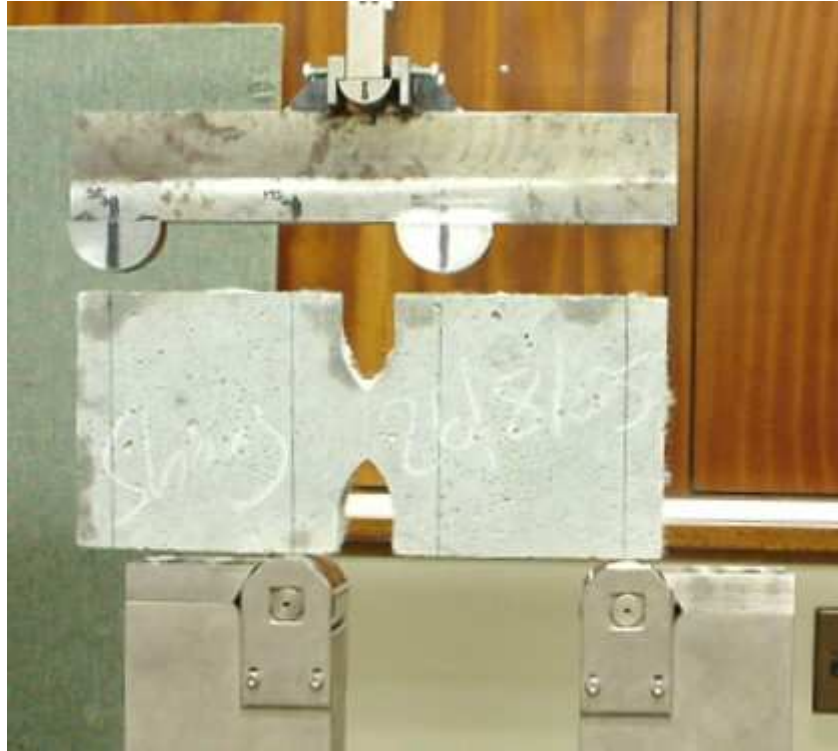
Figure 6.21 Experimental test setup for the Iosipescu shear test (Shang 2006).
