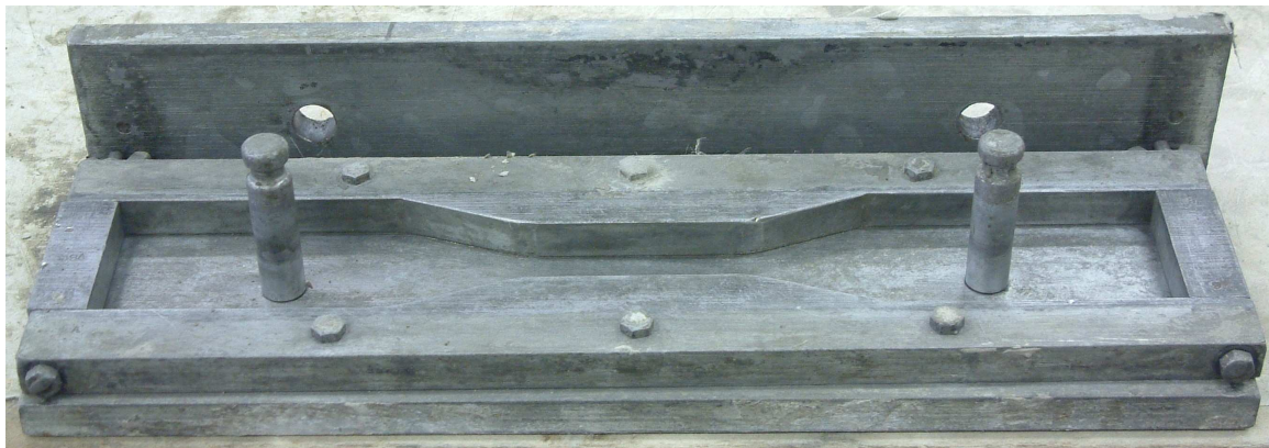
Figure 3.3 The steel mould for the flat dog bone specimens with the two removable studs.
